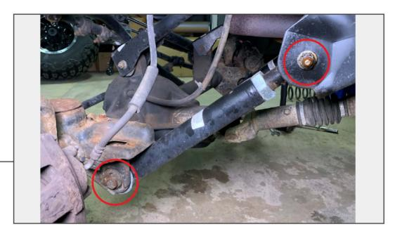
While supporting the axle, remove the (2) 21mm bolts holding the control arm to the vehicle. Remove the control arm from the vehicle.
