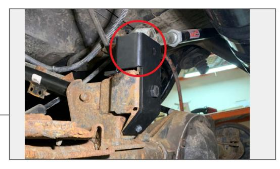
Reinstall the wheels and place the vehicle on the ground. Reinstall the track bar onto the axle using provided (1) M10x65mm bolt, lock washer, flat washer, and nut.
