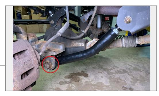
Install the adjustable control arm into the vehicle reusing original hardware. Be sure to reinstall the cams to adjust alignment.
