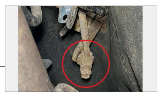
Test four wheel drive functionality. Adjust the linkage at the tail end of the transfer case linkage by loosening the screw using a 13mm socket and moving the adjuster where necessary to give the shifter more travel.
