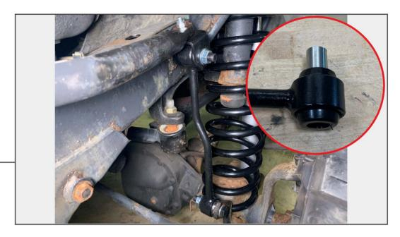
Using spray lubricant/grease and a hammer, tap the bolt sleeves into the front sway bar links. Using provided M12x65mm bolts, nuts, and washers, install the front sway bar links to the vehicle.
