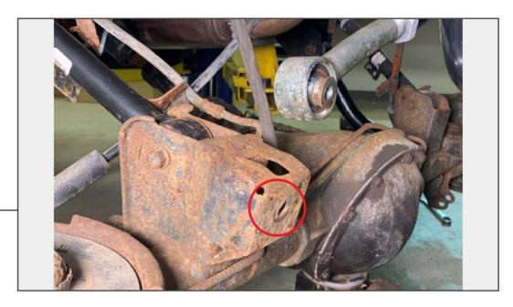
Slowly lower the axle down with the floor jack to provide enough space to remove the T-55 Torx bolt securing the track bar to the axle housing. Use a pry bar to separate the track bar from the axle.
