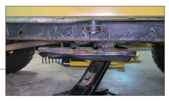
Remove (3) bolts on one side of the skid plate, then slowly lower the skid plate down approximately 2".
