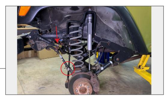
Remove the sway bar link bolt from the axle mount using a 15mm socket and a 18mm wrench. Remove the top nut on the sway bar link using a 15mm socket.
