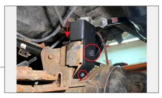
Install the provided track bar relocation bracket onto the axle housing using provided (1) M10x65mm bolts, lock washers, flat washers, and nuts, as well as (2)  $5/16 \times 1$ " bolts, washers, and lock nuts.
