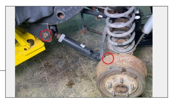
Loosen and remove the (2) 21mm control arm bolts from the vehicle. Remove the control arm from the vehicle.
