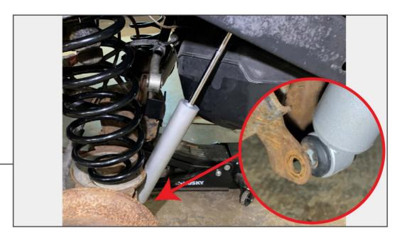
Note: Using an adjustable wrench, spread the lower shock mount sides apart if necessary to fit the shock absorber.
