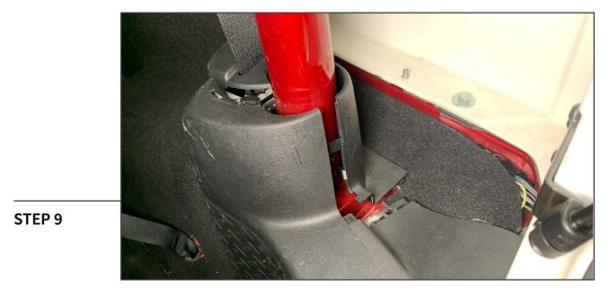
Carefully pry the trim panels apart. Remove the smaller panel to access the remaining 10mm nut.
