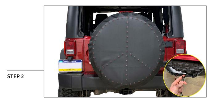
Center the cover on the tire, pull the draw string tight securing the cover to the tire.
