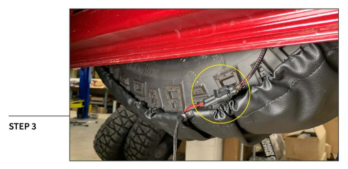
Connect the supplied wiring harness to the plug located at the bottom of the tire cover.
