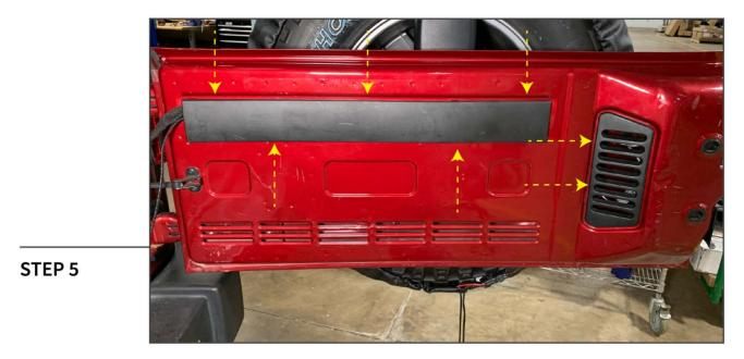
Using a soft pry tool, remove the (2) interior trim panels.
