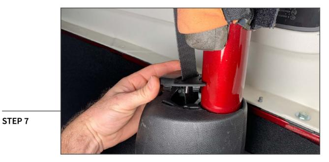
Using a soft pry tool, remove the seat belt trim bezel.
