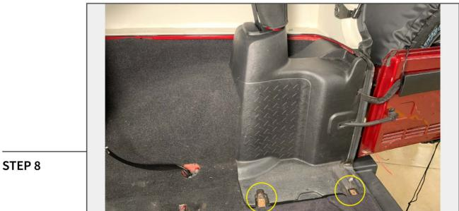
Using a T30 Torx bit, remove the (2) screws securing the trim panel to the vehicle.
