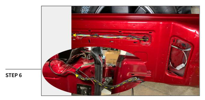
Locate and feed the wiring harness through the tailgate. Feed the wiring harness through the factory wire sheathing into the interior of the vehicle.
