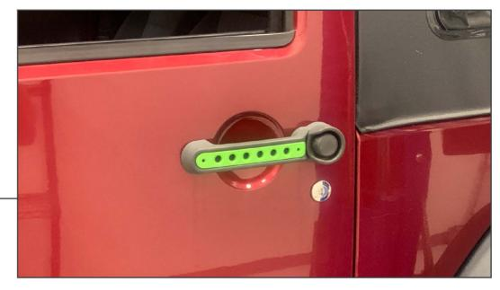
Install the door handle insert using the provided Phillips head screws.
