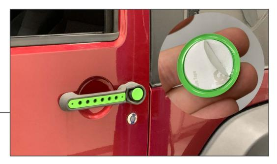
Peel back the tape backing from the push button covers. Press the covers onto the vehicle. Apply firm even pressure to ensure the proper adhesion. Repeat the process on the remaining door handles. Installation is now complete.
