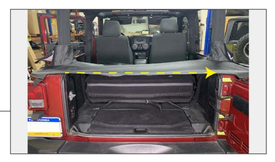
Slide the tailgate bar onto the tonneau cover. Place the tonneau cover onto the vehicle with the tonneau cover.
