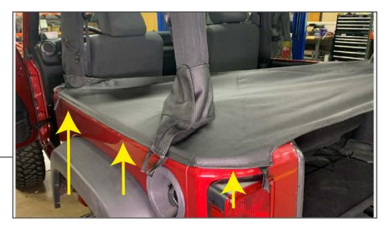
Tuck the sides of the tonneau cover under the lip of the vehicle's body. Use the pull straps for additional leverage. Repeat procedure to the opposite side.
