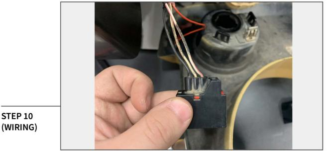
Using provided ScotchLocks, tap into the following wires for light functionality. Repeat installation on opposite side. Installation is now complete.
