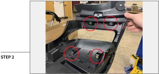
Begin assembling the new fender flare by inserting (4) Small U-Clips into the fender flare.
