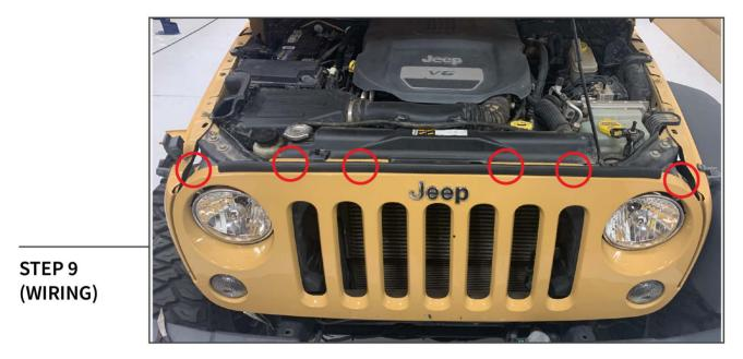
Remove grille from the vehicle by removing (6) push clips along the top. Firmly pull the grille away from the vehicle. Unplug the turn signal wiring harness from the light socket.
