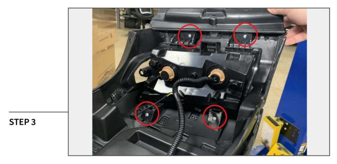
Install the turn signal lens into the fender flare using (4) Small Phillips Screws.
