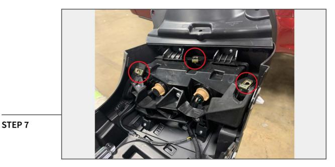
Install (3) M6 U-Clips into the Turn Signal Support Bracket. Fold the flap down, the secure with (3) M6 Phillips Screws.
