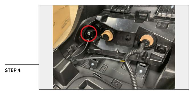
Install the marker light lens to the turn signal housing using (1) Large Phillips Screw. The lens gets inserted through the front of the fender flare. Plug in the marker light harness into the turn signal wiring harness.
