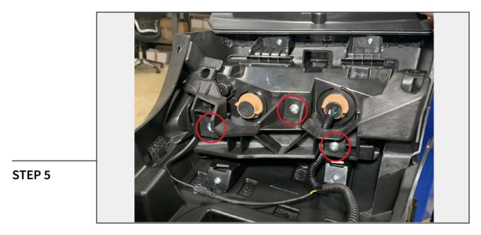
Install the Turn Signal Support Bracket to the fender flare using (3) Large Phillips Screws.
