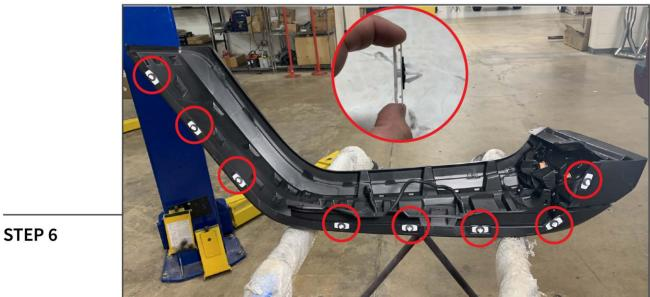
Install (8) Fender Clip Pads onto (8) Fender Clips, then slide them into the fender flare.
