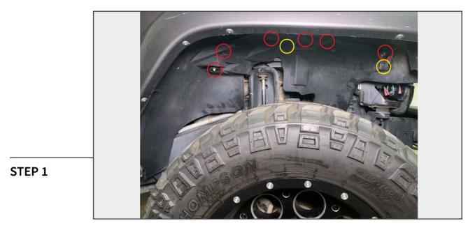
Remove (6) 10mm bolts and (2) push clips from the fender liner. Unplug the parking light connector. Firmly pull fender flare away from vehicle.
