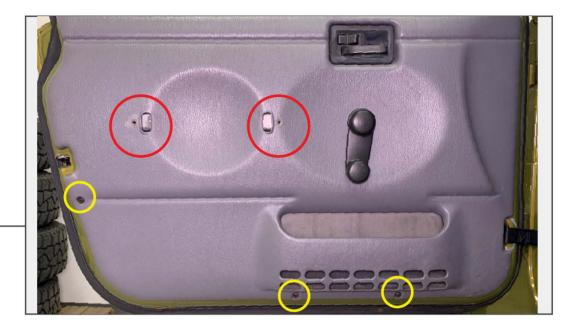
Remove (2) T-15 Torx screws from the door handle, and (3) Phillips screws from the bottom of the door panel. Remove the door handle from the vehicle.
