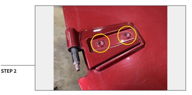
Remove (2) T-50 Torx bolts per hinge to remove the hinge from the door.
