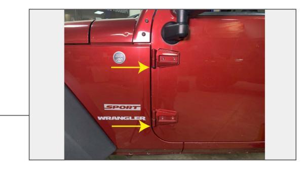
Remove door from vehicle by removing (2) T-50 Torx nuts from the bottom of the hinge. Unplug the door connector and release the limiting strap. Lift door away from vehicle.
