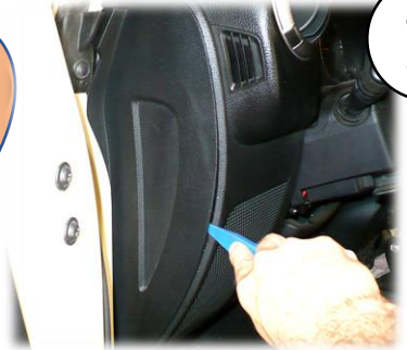
Use a mini plastic pry bar or thin flathead screwdriver and pop of Driver side dash side panel as shown. It's held on by several plastic clips and will simply snap back in place later on.
