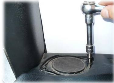
Remove two bolts for each tweeter with 7mm socket and ratchet.
