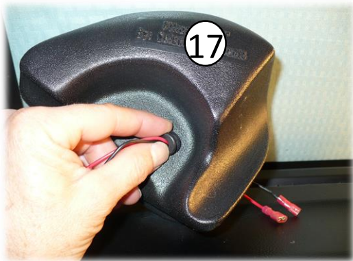
17 Remove poly-fill from pods for the moment. Run speaker terminals through small hole in back of each pod and seat grommet in hole by pushing it in and picking it through with your other hand.
