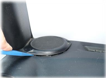
Pop off tweeter covers with plastic mini pry bar or thin flathead screwdriver.
