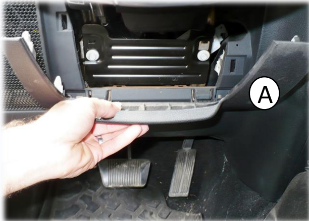
Give the panel under the steering wheel a tug, it'll pop right off.
