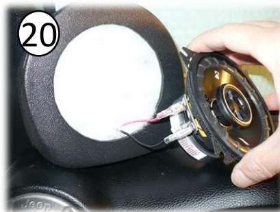
20 Replace the poly-fill, spreading it out inside the pods, making sure the wires are hanging out. Connect terminals to speaker. Large terminal is pos.+ and small terminal is neg.-
