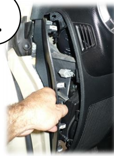
Use a mini plastic pry bar or thin flathead screwdriver and pop of Driver side dash side panel as shown. It's held on by several plastic clips and will simply snap back in place later on.
