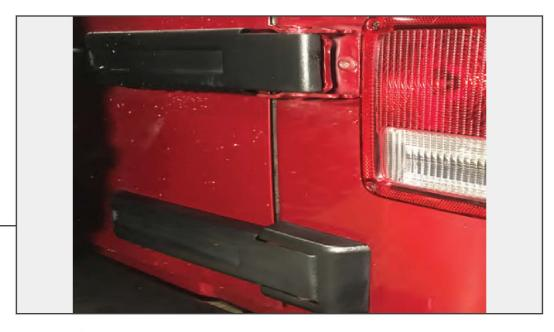
Clean the tailgate hinge surfaces prior to installation using alcohol wipes/isopropyl alcohol to ensure a secure bond.
