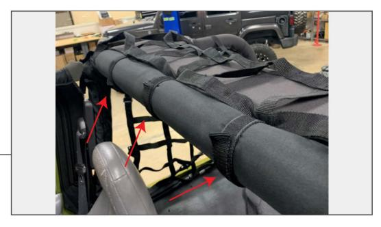
Loosely trap the central net into place starting with the roll bar in the center of the vehicle, then moving towards the side roll bars.
