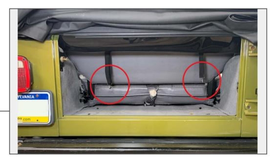
Drape the central net over the roll bar in the middle of the vehicle. Be sure the (2) hooks are located towards the rear of the vehicle as these will hook in the cargo area.
