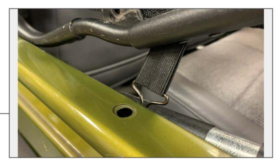
Tighten all the straps on each net to secure the cargo net into place. Attach the hooks at the bottom of the side nets to the vehicle above the quarter panel.
