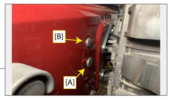
Insert (1) large plug into the tailgate in place of the third brake light grommet [A]. Insert (1) small plug into the tailgate in place of the spare tire bumper [B].
