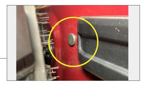
Insert (1) small plug into the tailgate in place of the spare tire bumper [B].
