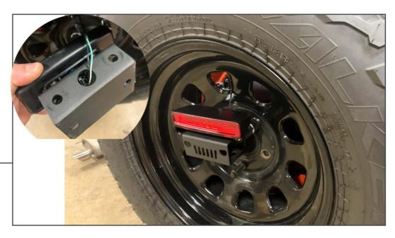
Feed the 3rd brake light wiring harness through the wheel. Plug the harness into the 3rd brake light. Then mount the 3rd brake light bracket to the upper mounting lug nuts using the supplied Allen bolts and washers.
