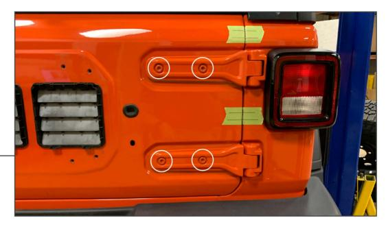
Using a T55 Torx bit, remove the (4) fasteners securing the tailgate hinge to the vehicle.
