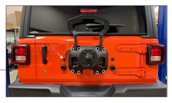
Pull the wiring harness through the tailgate. Using a 13mm socket, remove the (8) bolts securing the tire carrier to the tailgate.
