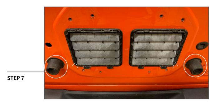
Remove the factory rubber bumpers. Using cutters, trim the factory tailgate vent.
