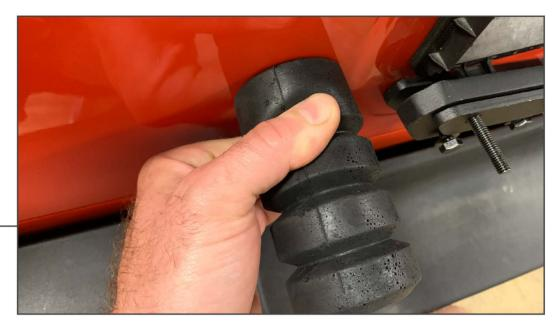
Firmly hold the base of the tire bumper and screw it into the tailgate. You must apply firm pressure while twisting the bumper clock-wise into the tailgate. .
