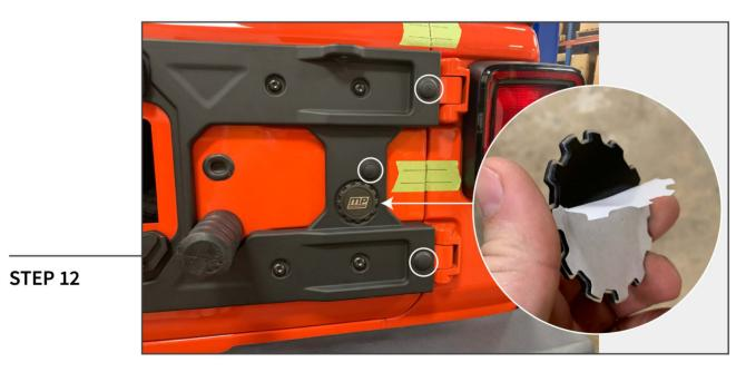
Peel off the tape backing from the MP Concepts logo and install as shown. Press the (3) plastic push pins into the (3) remaining holes.
