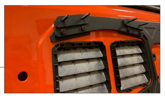
Secure the upper bracket and spacer to the vehicle using the supplied hex head bolts. Torque to 13 ft-lbs.
