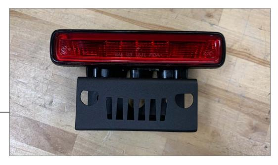
Install the 3rd brake light to the supplied bracket using the factory screws.
