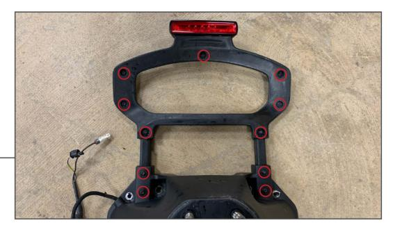
Using a T25 Torx bit, remove the 3rd brake light assembly from the factory tire carrier.
