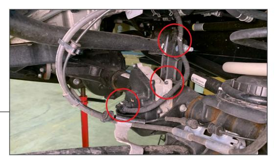
On the passenger side of the axle, disconnect the wiring and plug from the axle housing.
