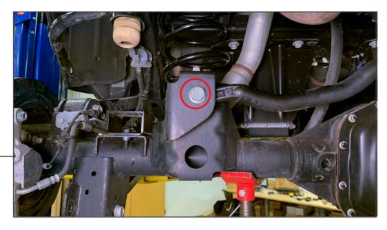
Loosely reinstall the factory track bar bolt. Do not fully tighten it at this time.
