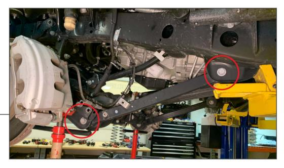
Using a 21mm wrench and 24mm socket, loosen and remove bolts securing the lower control arms to the vehicle.
