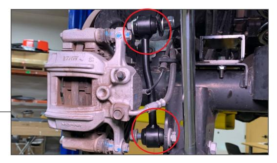
Loosely Install the longer of the provided end links. Use the provided M12x1.25 70mm bolts, (2) washers, and (1) Lock nut per side for the upper mount. Reuse the factory hardware for the lower mounts. Repeat this process on both sides of the axle.
