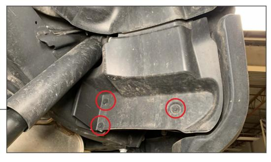
Using a 8mm socket, remove the (3) bolts securing the bottom portion of the fender liner to the vehicle. This will allow access to the upper shock bolt.
