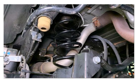
Install the rears springs. Reuse the factory upper and lower spring isolators. Carefully raise the rear axle.
