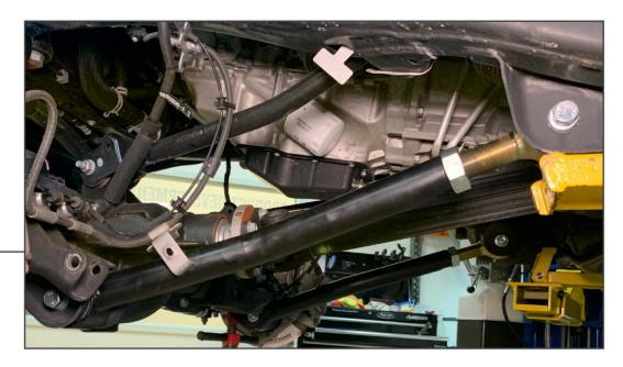
Loosely install the adjustable lower control arms so the gold end of the arm mount to the chassis. Do not fully tighten any mounting hardware until Step 28. Mount the brake line bracket to the lower control arm with the factory nut.
