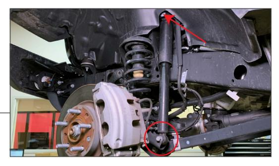
Using a 18mm socket to remove the upper shock bolt. Then, use a 18mm wrench and socket to remove the lower bolt. Hold the shock while removing the mounting hardware so that it doesn't fall off the vehicle.
