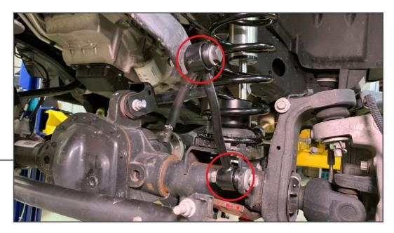
Loosely Install the shorter of the provided end links. Use the provided M12x1.25 70mm bolts, (2) washers, and (1) lock nut per side for the upper mount. Reuse the factory hardware for the lower mounts. Repeat this process on both sides of the axle.
