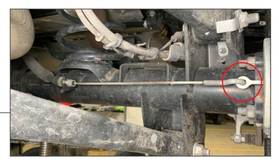
Ensure the brake is not applied prior to removing the cable. On the front of the axle tube, locate and disconnect the emergency brake cable. Use a pair of pliers to carefully twist the cable end off of the brake mechanism.
