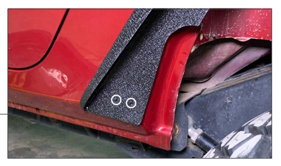
With the fender flares secured to the vehicle, finish by installing the (2) self-tapping screws at the front of the rear fender.
