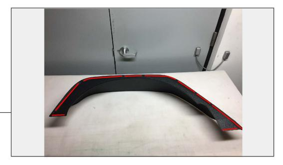
Install the supplied foam to the fender before installation.
