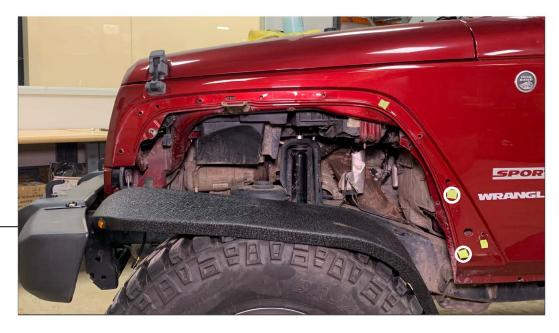
Drill through the outer and inner fender in the locations circled above. These locations will receive spacers and M8 bolts. Paint any exposed metal with touch up paint or clear nail polish.
