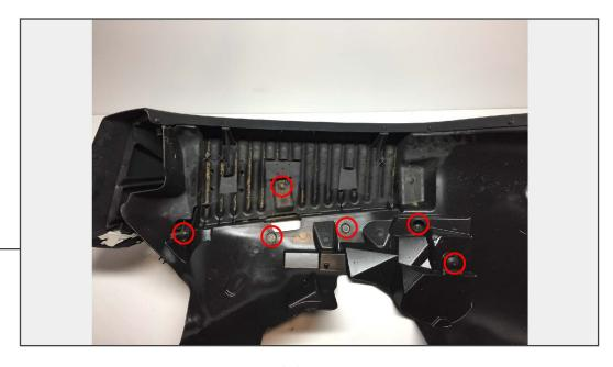
Begin by removing the factory fender liners, there are (5) 10mm bolts. Disconnect the factory marker light harness from the light. Remove the factory fender flare by firmly pulling it away from the vehicle, starting from the front of the fender and working towards the rear. Some of the factory plastic clips may break when removing the fenders this is normal. The clips are not required for installation of the new flares.
