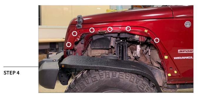
Drill the (6) holes circled above to 25/64". Paint any exposed metal with touch up paint or clear nail polish. Using the provided rivnut tool, install the supplied rivnuts.
