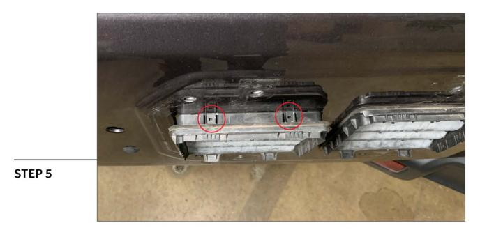
Using a soft pry tool, remove the factory tailgate vents.
