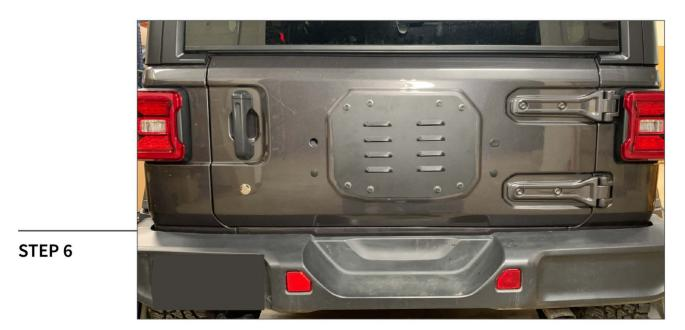
Install the spare tire delete using the factory hardware removed in Step 5. Installation is now complete.
