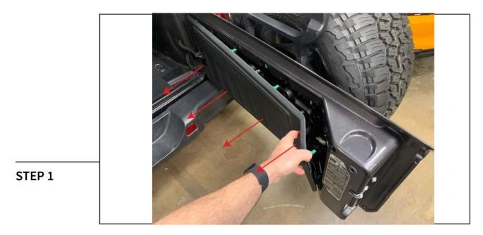
Begin by opening the tailgate to gain access to the tailgate trim panel. Using a soft pry tool, pry the trim panel away from the tailgate. Any of the green clips that remain in the tailgate will need to be removed and press back onto the trim panel prior to re installation.
