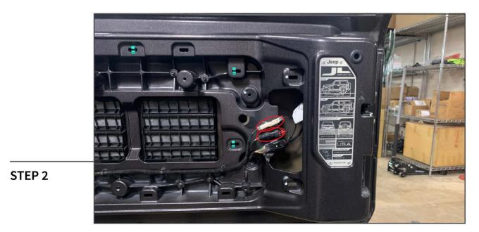
Remove the 3rd brake light and reverse camera wiring connections. Depress the tab and pull the plugs apart.
