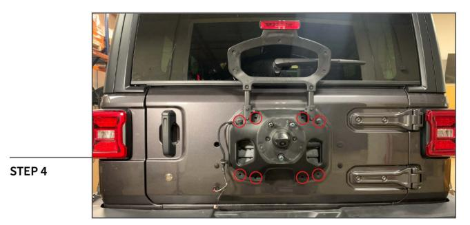
Pull the wiring harness through the hole in the tailgate. Using a 13mm socket, remove the (8) bolts securing the factory tire carrier to the vehicle.
