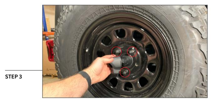
Using a T40 torx wrench unlock the reverse camera trim panel and remove it from the vehicle. Using a lug wrench, remove the (3) lug nuts securing the spare tire to the vehicle. Remove the tire.
