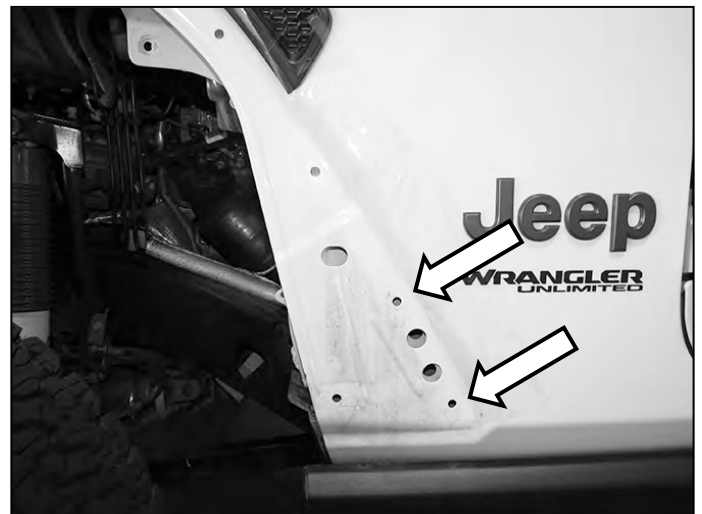
(Fig 8) Use a 25/64" drill bit to open holes up slightly for Threaded Insert installation (see Fig 7)
