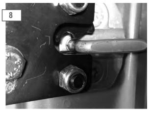
Align the door latch with the striker using the latch spacers as seen above. \*\*Note: Spending extra time aligning the latch to the striker will result in a smoother feel when opening and closing the door.
