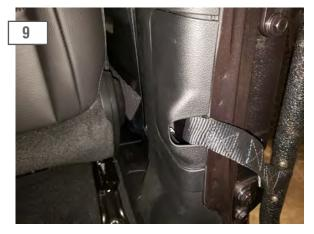
Install the door strap from the HD Adventure Door to the chassis mount. Reinstall the trim panel.
