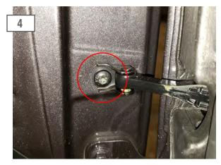
Locate, and remove the T40 torx bolt securing factory door hinge stop. Lift the door up to remove it from the vehicle. Then reinstall the factory T40 torx bolt as a place holder to ensure it doesn't get lost.
