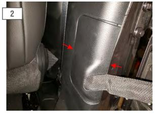
Slide the front seat forward to access the interior trim panel. Using a panel removal tool, pry the panel off. \*\*Note: The panel has indents on the sides, pry from those indents.
