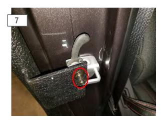
Loosely install the door latch using the M6x1.0x25mm screws, flat washers, and lock washers.
