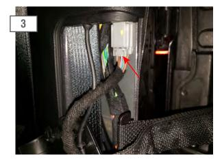
Roll down the windows so that the door is easier to handle while removing it from the vehicle. Unplug the connector. Slide the hinge strap off the chassis mount.
