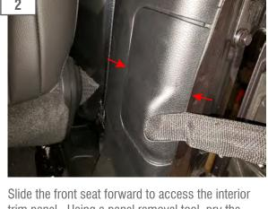
Slide the front seat forward to access the interior trim panel. Using a panel removal tool, pry the panel off. \*\*Note: The panel has indents on the sides, pry from those indents.
