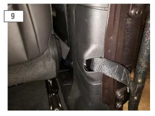
Install the door strap from the Tubular Door to the chassis mount. Reinstall the trim panel.
