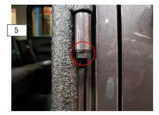
Install the new door, you may need to use a rubber mallet to seat the door all the way onto the hinge. Use the supplied M8 nut and washer to secure the door to the hinge.
