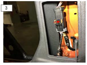
Roll down the windows so that the door is easier to handle while removing it from the vehicle. Unlock the red locking mechanism and then unplug the connector. Slide the hinge strap off the chassis mount. Lift the door up to remove it from the vehicle.
