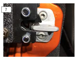
Align the door latch with the striker using the latch spacers as seen above. \*\*Note: Spending extra time aligning the latch to the striker will result in a smooth feel when opening and closing the door.
