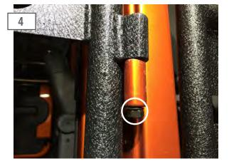
Install the tubular door, you may need to use a rubber mallet to seat the door all the way onto the hinge. Use the supplied M8 lock nut and flat washer to secure the door to the hinge.
