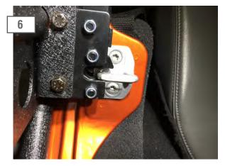
Loosely install the door latch using the M6x1.0x25mm screws, flat washers, lock washers, and (1) M6 dual nut plate.
