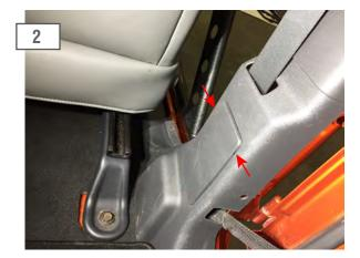
Slide the front seat forward to access the interior trim panel. Using a panel removal tool, pry the panel off. \*\*Note: The panel has indents on the sides, pry from those indents.
