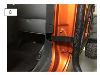
Install the door strap from the tubular door to the chassis mount. Reinstall the trim panel. Installation is now complete.
