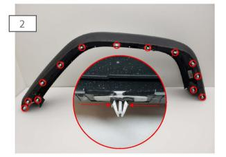
The fender has (13) plastic push clips. Carefully depress the clips using a trim panel removal tool. Then remove the fender from the vehicle.
