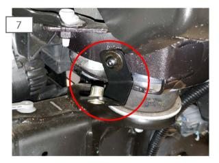
Attach the lower body bracket to the speed clip that was installed in the last step using (1) M10x1.50x25mm Allen bolt, lock washer, and flat washer.
