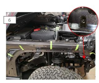
Locate the lower body mount, and insert the (1) speed clip.
