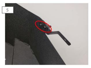
Install the right side bracket to the rear upper right portion of the inner liner using (2) M10x1.50x25mm Allen bolts, large flat washers, small flat washers, and lock nuts.
