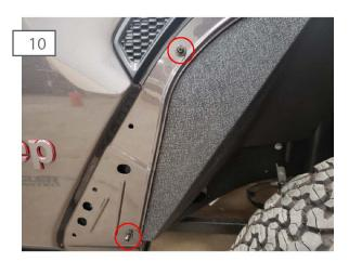
Align the rear portion of the fender liner with the holes of the factory fender flare. Attach the rear portion of the fender liner to the body using (2) M10x1.50x25mm Allen bolts, lock washers and flat washers.
