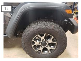
Reconnect the fender flare wiring harness. Align the fender flare with the factory hole locations and gently press the fender flare in to secure to the body. Then reinstall the (3) 10mm bolts from Step 3. Repeat steps 1-11 for the opposite side. Installation for the front is now complete.
