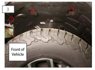
Located and remove the (3) 10mm screws securing the front portion of the front fender liner in place. Then fully remove the fender liner from the vehicle.
