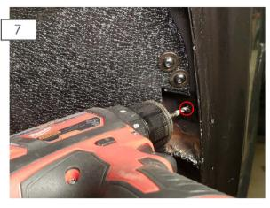
Beginning from right to left, press the upper mounting bracket against the inner body of the vehicle. Using a drill & 3/16" drill bit, carefully drill the mounting holes. Apply touch up paint to prevent corrosion.
