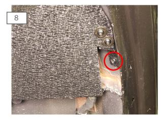
Once 3/16" holes are drilled, secure the mounting brackets to the body of the vehicle using (1) Phillips head screw and small flat washer. Repeat for all (3) upper brackets.
