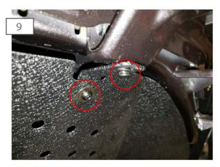
Attach the upper fender bracket to the fender mount using the (1) M10x1.50x25mm Allen bolt, lock washer, flat washers, and nuts. Then attach the upper portion of the fender liner to the upper fender bracket using (1) M10x1.50x25mm Allen bolt, lock washer, and flat washer.
