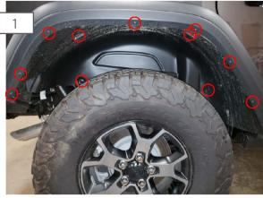
Begin by removing the factory fender liner by removing the plastic pop rivets, (2) 10mm screws, and (2) push clips located above.
