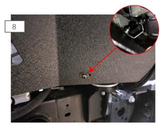
Hold the inner fender liner up to the wheel well. Attach the lower front portion of the inner fender liner to the lower body bracket using (1) M10x1.50x25mm Allen bolt, lock washer, and flat washer.
