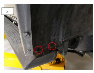
Using a trim panel removal tool, locate and remove the (2) lower push clips securing the back portion of the front fender liner in place.
