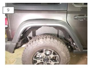
Align the fender flare with the factory hole locations and gently press the fender flare in to secure to the body. Repeat steps 1-8 for the opposite side. Installation for the rear is now complete.
