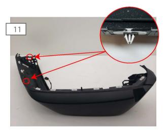
Remove the (2) plastic push clips shown in the picture above using a flat head screw driver. \*\*Note: These locations are now being used by the rear portion of the fender liner hardware.
