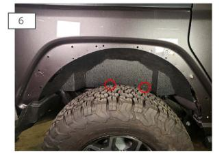
Hold the inner fender liner up to the wheel well. Align the inner fender liner to the lower factory body holes, and mount using (2) M10x1.50x25mm Allen bolts, large flat washers, small flat washers, and lock nuts.
