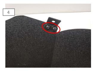
Install the middle bracket to the middle upper portion of the inner liner using (2) M10x1.50x25mm Allen bolts, large flat washers, small flat washers, and lock nuts.
