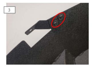
Install the left side bracket to the rear upper left portion of the inner liner using (2) M10x1.50x25mm Allen bolts, large flat washers, small flat washers, and lock nuts.
