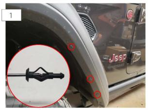
Begin by removing the factory fender liners by removing the (3) plastic pop rivets located above by using a small Phillips head screw driver and pushing the center of the rivet through.
