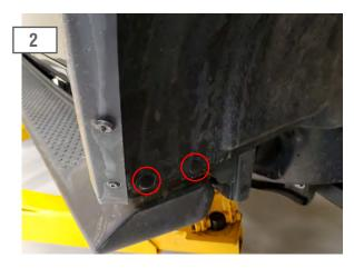
Using a trim panel removal tool, locate and remove the (2) lower push clips securing the back portion of the front fender liner in place.
