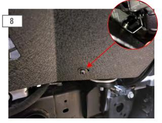
Hold the inner fender liner up to the wheel well. Attach the lower front portion of the inner fender liner to the lower body bracket using (1) M10x1.50x25mm allen bolt, lock washer, and flat washer.
