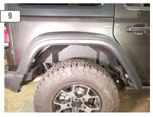
Align the fender flare with the factory hole locations and gently press the fender flare in to secure to the body. Repeat steps 1-8 for the opposite side. Installation for the rear is now complete.
