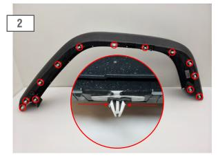
The fender has (13) plastic push clips. Carefully depress the clips using a trim panel removal tool. Then remove the fender from the vehicle.
