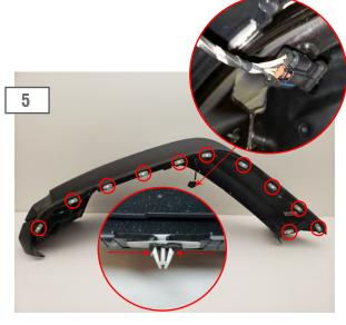
Locate, and unplug the fender wiring plug connector. Then locate and carefully depress the (11) plastic push clips using a trim panel removal tool, and remove the fender from the vehicle.
