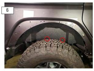
Hold the inner fender liner up to the wheel well. Align the inner fender liner to the lower factory body holes, and mount using (2) M10x1.50x25mm allen bolts, large flat washers, small flat washers, and lock nuts.
