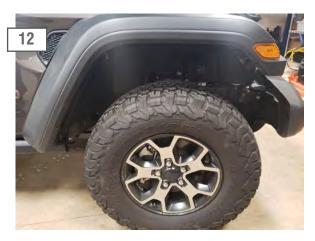
Reconnect the fender flare wiring harness. Align the fender flare with the factory hole locations and gently press the fender flare in to secure to the body. Then reinstall the (3) 10mm bolts from Step 3. Repeat steps 1-11 for the opposite side. Installation for the front is now complete.
