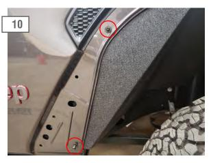
Align the rear portion of the fender liner with the holes of the factory fender flare. Attach the rear portion of the fender liner to the body using (2) M10x1.50x25mm allen bolts, lock washers and flat washers.
