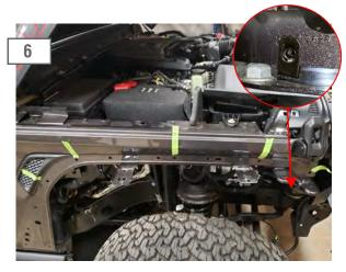
Locate the lower body mount, and insert the (1) speed clip.
