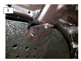
Attach the upper fender bracket to the fender mount using the (1) M10x1.50x25mm allen bolt, lock washer, flat washers, and nuts. Then attach the upper portion of the fender liner to the upper fender bracket using (1) M10x1.50x25mm allen bolt, lock washer, and flat washer.
