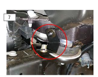
Attach the lower body bracket to the speed clip that was installed in the last step using (1) M10x1.50x25mm allen bolt, lock washer, and flat washer.
