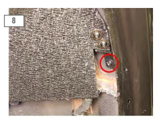
Once 3/16" holes are drilled, secure the mounting brackets to the body of the vehicle using (1) Phillips head screw and small flat washer. Repeat for all (3) upper brackets.
