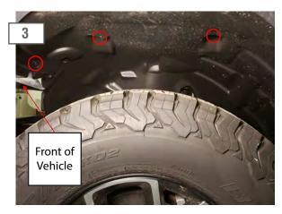
Located and remove the (3) 10mm screws securing the front portion of the front fender liner in place. Then fully remove the fender liner from the vehicle.
