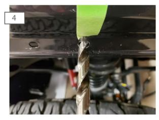
Using a 25/64" drill bit and drill, drill out the pre-determined holes from Step 3.
