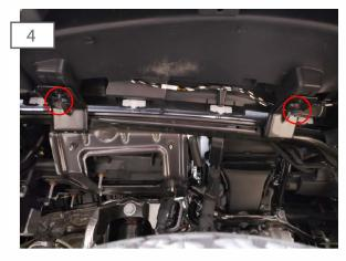
Locate, and remove the (2) 10mm screws holding the fender to the fender brackets.
