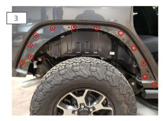
Hold the fender up to the body of the vehicle to determine which holes will need to be drilled for the installation of the provided rivnuts.
