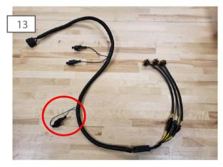
D38 Fender Flares w/ (3) LED Marker Lights to Factory LED Plug in the supplied "T" harness between the chassis plug and the factory fender plug. Connect the (3) plug ends to the fender LED lights. For vehicles with factory LED Lights, connect the weather-tight plugs into the (2) black wire connectors as they will not be used. Plug the (2) green wire connectors together. \*\*Note: If optional D38 Grille is not being installed, proceed to Rear Fender Install.
