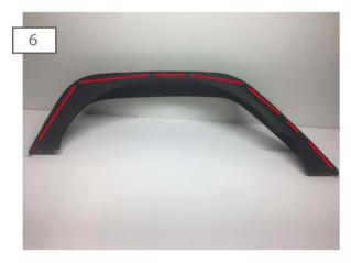
Install the supplied foam to the fender before installation as shown above.
