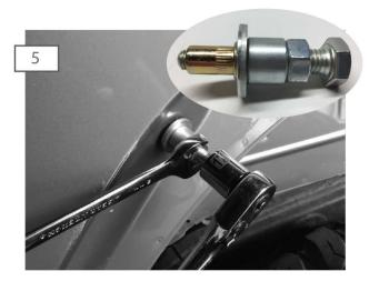
Insert the rivnut into the pre-drilled hole. Thread the rivnut tool onto the rivnut. Using a 16mm wrench, hold the nut in place while turning the head of the bolt with a 17mm ratchet. Tightening the bolt will clamp the rivnut against the sheet metal. \*\*Note: Do not over tighten the rivnut. Doing so can pull the threads out of the insert.
