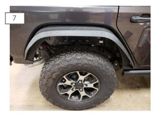
Secure the fender to the vehicle using the M6x1.00 25mm bolts with the supplied washer, and lock washer on all mounting locations containing rivnuts. Installation is now complete.
