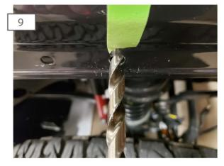
Using a 25/64" drill bit and drill, drill out the pre-determined holes from Step 8.
