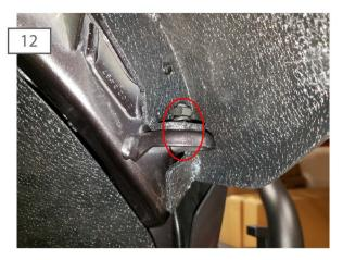
Secure the front section of the fender to the fender bracket using the (1) M8x1.25x25mm bolt, flat washer, lock washer and nut.
