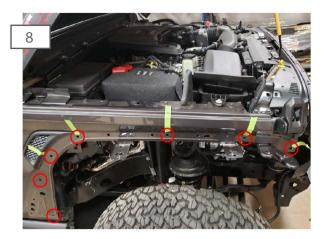
Hold the fender up to the body of the vehicle to determine which holes will need to be drilled out. The holes shown above will be drilled for the installation of provided rivnuts.
