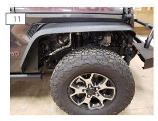
Secure the fender to the vehicle using the M6x1.00 25mm bolts with the supplied washer, and lock washer on all mounting locations containing rivnuts.
