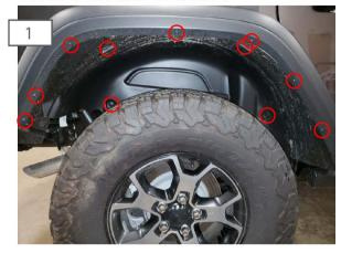
Begin by removing the factory fender liners by removing the plastic pop rivets, (2) 10mm screws, and (2) push clips located above.
