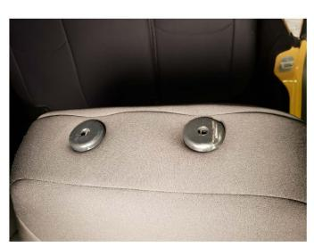
**Step 3\\**Once the upper portion of the seat cover is installed, tuck the seat cover under the tabs for the headrest guides.
