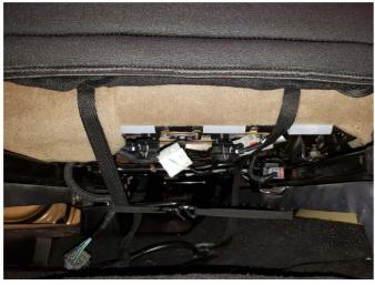
**Step 5\\**Connect the (2) front to back and (1) side to side clips to secure the seat cover to the lower portion of the seat. Then pull tight on the strip to ensure the seat cover is tight to the seat.
