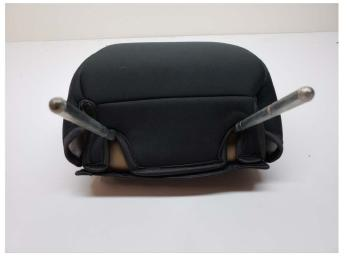
**Step 1\\**Begin by removing the headrest on each side, and sliding over the new headrest covers. Secure the cover to the headrest by velcroing them in place.
