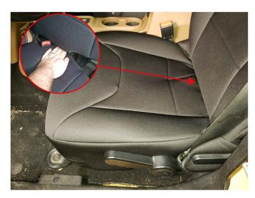
**Step 4\\**Install the lower portion of the seat cover to the seat. Tuck the two buckles through the upper and lower seat joint.
