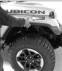
Step 2. Take hold of the front part of the flare and firmly pull up to release the hidden factory mounting clips as shown above. Move to the center of the flare then rear of the flare pulling firmly up and back. You will hear a clicking sound as the clips are released as shown above. Repeat steps 1-4 above for other side.
