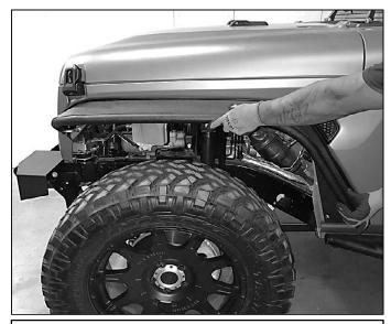
Step 1. Locate and place supplied driver fender flare (A) onto jeep as shown. Line up the fender flare holes with the jeep holes.
