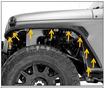
Step 2. Place supplied M8x1.25x20mm button head bolt (D) with supplied M8 flat washer (C) through the hole in the fender and through the holes on the vehicle fender. Start a supplied M8x1.25 flange nut (E) at the end of bolt. **Do not tighten bolts at this time.**
