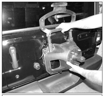
Step 6. Remove factory tire carrier from vehicle. Set factory tire carrier aside in a protected area.
