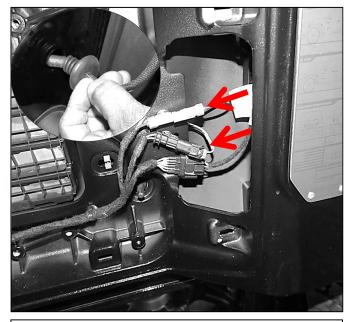
Step 4. Locate and disconnect the 3<sup>rd</sup> brake light and back up camera. Firmly press down on the Mate-m-lock plug. Remove brake light plug with plastic rivet removal tool or similar tool. Feed 3rd brake light/backup camera plug back through the swing gate.
