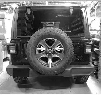
Step 2. Using a 22mm socket remove all three factory lug nuts holding the spare tire in position. Remove factory spare tire from the vehicle. Set factory hardware and spare tire aside for later use.
