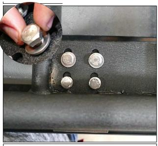
Step 2. Working on the top side of the mounting bracket . Place a supplied M8x1.25x25mm hex head bolt with supplied M8 flat washer through the holes in the roof rack onto the holes on the mounting bracket. Tighten down using a 13mm socket. Repeat step for remaining bolts. Repeat step for 1-2 for remaining rear mounting brackets. Repeat step 1-2 for other side.
