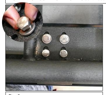
Step 2. Working on the top side of the mounting bracket (E). Place a supplied M8x1.25x25mm hex head bolt (H) with supplied M8 flat washer (M) through the holes in the roof rack onto the holes on the mounting bracket. Tighten down using a 13mm socket. Repeat step for remaining bolts. Repeat step for 1-2 for remaining
