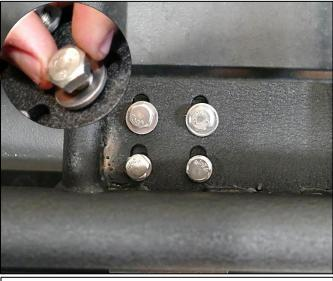
Step 4. Working on the top side of the large mounting bracket (T). Place a supplied M8x1.25x25mm hex head bolt (H) with supplied M8 flat washer (M) through the holes in the roof rack onto the holes on the mounting bracket. Tighten down using a 13mm socket. Repeat step for remaining bolts. Repeat step for 1-2 for remaining rear mounting brackets. Repeat step 1-2 for other side.
