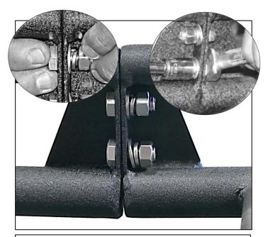
Step 3. Place supplied M6x1.0x25mm hex head bolt (J) through the holes in the front rack piece (C) and through the holes in the center rack piece (B). Place a supplied M6 flat washer (O) and supplied M6 split washer (R) at the end of bolt. Start a supplied M10x1.5 hex head nut at the end of bolt. Tighten down using a 5/8 socket and 5/8 wrench. Repeat step for remaining bolt. Repeat step for other side.
