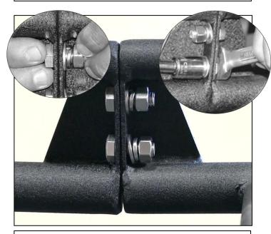
Step 3. Place supplied M6x1.0x25mm hex head bolt (J) through the holes in the center rack piece (B) and through the holes in the rear rack piece (A). Place a supplied M6 flat washer (O) and supplied M6 split washer (R) at the end of bolt. Start a supplied M6 hex head nut at the end of bolt. Tighten down using a 5/8 socket and 5/8 wrench. Repeat step for remaining bolt. Repeat step for other side.
