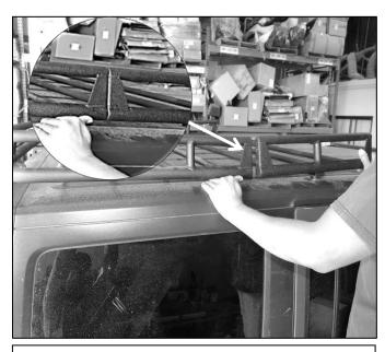
Step 2. Place supplied center rack piece (B) onto Jeep as shown above. Line up the center rack piece holes with the holes in the rear rack piece.
