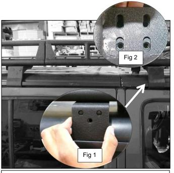
Step 3. Place supplied large mounting brackets (S) towards the front of the Jeep as shown above fig 1. Line up the top mounting holes with the roof rack mounting holes as shown in fig 2.
