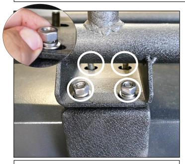
Step 2. Place supplied M8 flat washer (M) and supplied M8 split washer (N) onto the end of bolt. Start a supplied M8x1.25 hex head nut (L) at the end of bolt. Repeat step for remaining nuts. Tighten down using 13mm socket.
