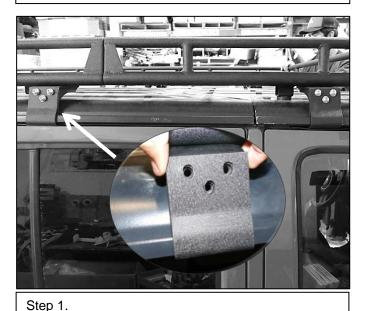
Open Jeep door. Place supplied small clamp (D) onto mounting bracket (E) as shown above. Secure clamp into place by placing a supplied M8x1.25x25mm Allen head bolt (I) with supplied M8 flat washer (M) and supplied M8 split washer (N) through the holes in the clamps onto mounting bracket holes. Repeat step for remaining bolts. Tighten down all hardware using a 3/16 Allen key wrench. Repeat step for remaining clamps. Repeat step for other side.
