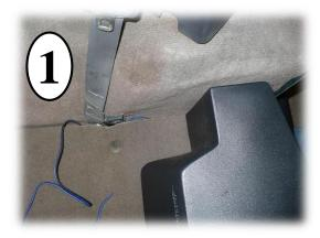
Place the pod in cargo area passenger side (we'll fine tune exact positioning later) and start to tuck speaker wire under carpet. Make sure pod isn't resting on wire. Pop wires up through carpet at your amplifier (a small slit in the carpet at the appropriate are will do) and connect wires to amp.
