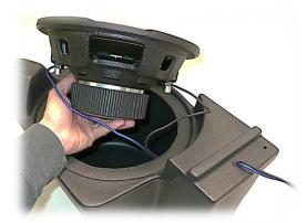
Install rubber grommet in underside hole and run speaker wires through to connect to your subwoofer. Place sub in pod and gently pull any excess speaker wire back through the grommet. This may take a few attempts... you want it slightly loose but excess wire could vibrate if it's touching the pod walls.
