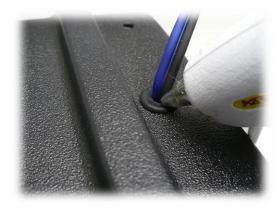
Use a glue gun (or similar medium) to plug any remaining air space around speaker wires as they exit the grommet to ensure an air-tight seal (air escaping could make a whistling noise on bass notes.
