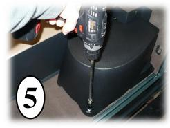
This screw first. Sheet metal is **THIN!** Don't overtighten any of the (3) screws!!
