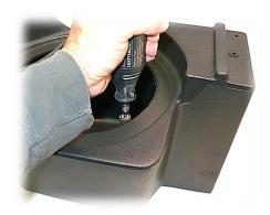
You may have to cut the subwoofer hole larger to accept your particular sub; easily done with a rotary cut-out tool and either a spiral drill bit or even a sanding drum such as used with a Dremel® rotary tool. (The pre-cut hole is about 9" diameter so it can work with subs that need smaller cutout diameters).
