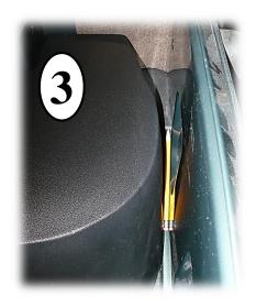
Close tailgate. Note pencil in photo. The pod Installs very close to the tailgate (in TJ's) and the lower section where the subwoofer is is the point that comes closest to the tailgate. **Photo is in a TJ**. Earlier CJ7 and YJ Jeeps have a slightly larger cargo area so the pod won't be as close to the tailgate as this. Once the pod is exactly where you want it, open the tailgate And we'll look at attaching pod to floor.
