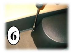
This screw next. Note Intsa-trunk wall in photo. Drill extension would contact it, but no need to remove the wall if you have one.
