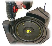
Use (8) provided black subwoofer screws to affix sub to pod, *starting* with a drill w/ phillips bit....
