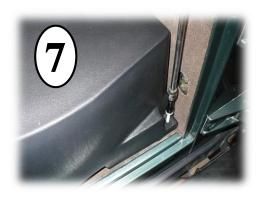
Final screw. After hand-tightening, push the included black screw caps over top of each screw. Time for sound tests and adjustments of your radio and amp settings.
