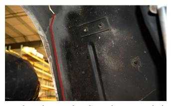
**15. Cut along the traced cut-line** with a pneumatic body saw, reciprocating saw, cut-off wheel or other appropriate cutting tool.
