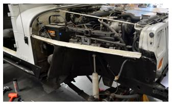
19. Note the remnants of the stock fender bracing where the fender attaches to the grille, near the top, as shown in the photo below. These will need to be ground flush and smoothed out.
