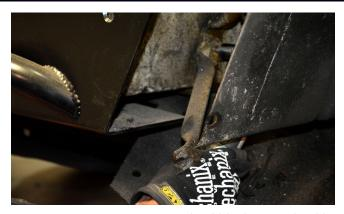
18. At this point your work should look somewhat like the photo below, with only the inner fender and a narrow strip along the top of the outer fender remaining. NOTE: your stock inner fender will NOT be attached to the Jeep's tub at this time—at this point in the installation process it will be unsupported except by the accessories bolted to it. This is normal. It will regain its rigidity once the DeFender™ has been installed.
