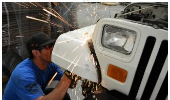
14. Toward the back, from underneath, notice that the rear of the inner wheel well continues downward from where you had cut through the top surface of the fender. You will want to cut downward from the point of the top-surface cut, continue as close to the outer sheetmetal skin as possible. You may be limited by your cutting tool with regards to how close to the outer sheetmetal you can cut. Mark a cut line, trying to leave as much of this inner wheel well as possible.
