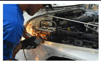
**12. When cutting along the front** portion near the grille, be careful not to damage the grille with the cutting tool. This is why the spacer inserted between the fender and the grille is important.
