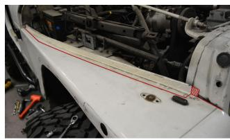
10. Continuing at the front of the fender, continue the cut line along the front of the fender adjacent to where it meets the grille. Continue the cut line downward until it reaches the edge of the fender. Place a rag or other suitable object between the fender and the grille to space it apart to gain access to the cut line with your cutting tool.
