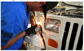
**13.** Once the outer sheetmetal is cut, you will need to go underneath the fender to finish some of the cuts. At the front of the fender, you may need to finish cutting through the thick metal hood latch support from the underside.
