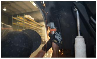
16. All of the major cutting is now complete, however you may find that you need to do further cutting at various inner flanges and corners, in order to fully free the cutaway portion of the fender. Once this has been done, lift the cut portion away and set it aside.
