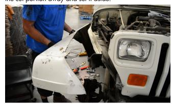
17. There may be a fender support bar behind the inner wheel well, that braced the fender to the firewall. Remove it if the material it had been attached to has been cut away.
