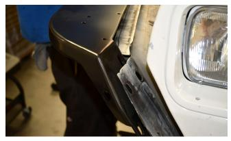
**24. Use the OE hardware to** bolt the DeFender<sup>™</sup> to the firewall and to the grille. Leave the hardware somewhat loose until both DeFenders <sup>™</sup> are installed to this point in the instructions. On CJ's, the headlight bezel and assembly will need to be removed to access the top nut (this is the second hole down from the top, and not an original fender mounting hole which is now blocked by the new DeFender<sup>™</sup>).
