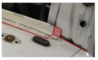
9. At the back of the fender, closer to where it joins the firewall, trace a line that begins 1/4" from the vertical flange and continues forward, parallel to the outside edge of the fender, to where it joins with the previous line. The resulting cut line should look like the one in the photo below.
