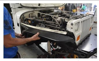
23. Ensure that the 1-1/4" wide strip of remaining material from the original fender is under the top surface of the DeFender™, and that the original part of the fender that bolted to the side of the grille is sandwiched between the corresponding part on the DeFender™, and the side of the grille, as shown in the photo below. Also make sure the sheetmetal at the back of the inner wheel well is positioned behind the wheel well mounting tabs on the DeFenders™.
