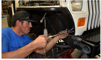
**25.** Once both DeFenders<sup>™</sup> are loosely installed, tighten all mounting hardware. Check and adjust alignment
