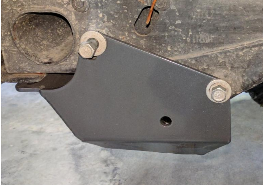
Figure 3. Synergy Steering Box Skid Installed with First Two Bolts (2005 Model Shown)
