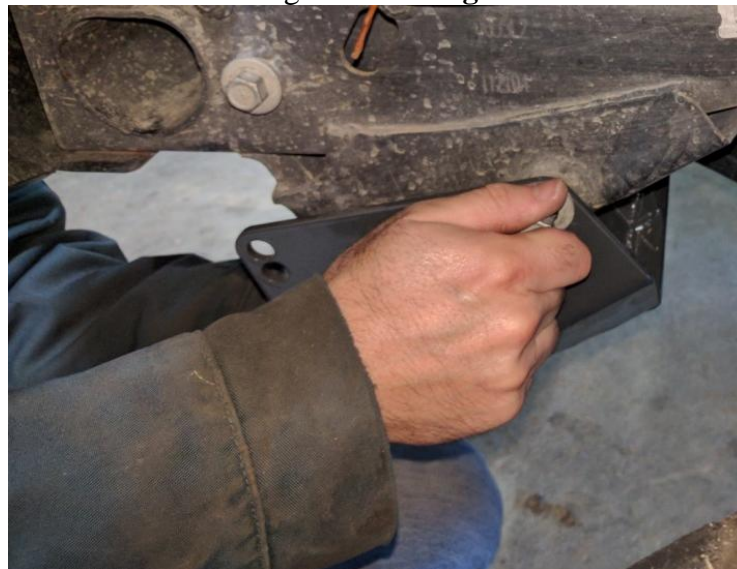
Figure 2. Installing First Bolt in Steering Box Brace
