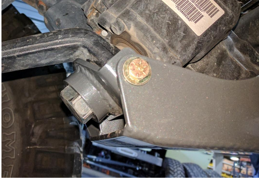
Figure 5. Sector Shaft Brace Installed
