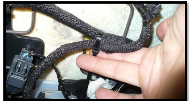
A cable tie can hold the excess wire lengths to the spring work of the seat bottom, ( check for full seat slide ability front to back ).
