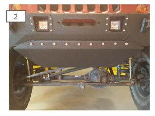
Install the skid plate to the bumper using the supplied (9) M8 x 1.25 x 25mm button head bolts, nuts, and washers. \*\*Note: Long extension may be required for inner nuts.
