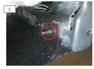
Install the skid plate to the chassis using the supplied (2) M8 x 1.25 x 40mm hex head bolts, lock washers, large washers, and nuts.
