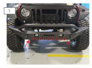
Identify the skid plate mounting locations as shown above.
