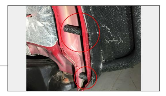
Install the supplied spacers between the inner and outer fenders using the M8 x 1.25 120mm bolt for the long spacer and the M8 x 1.25 65mm bolt for the shorter spacer.
