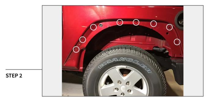
To install the supplied rivnuts, start by enlarging the (8) factory holes circled above using a 23/64" drill bit. Treat any exposed metal with touch up paint or clear nail polish.
