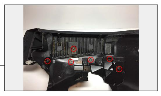
Begin by removing the factory fender liners, there are (5) 10mm bolts. Disconnect the factory marker light harness from the light and zip tie it out of the way. Remove the factory fender flare by firmly pulling it away from the vehicle, starting from the front of the fender and working towards the rear.
