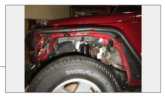
Install the Barricade Flat Fenders using the supplied M8 x 1.25 25mm long allen bolts, install the forward most (5) bolts first. Loosely install all hardware before fully tightening bolts to ensure proper bolt hole alignment.
