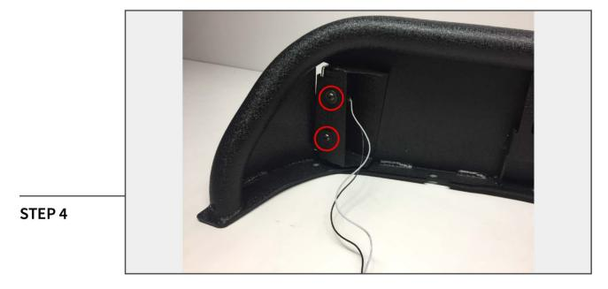
Mount the light/light bracket assembly to the fender using the supplied allen bolts and washers.
