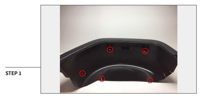
**REAR FENDER FLARE INSTALLATION:** Using a flat head screw driver or trim panel removal tool, remove the (5) push clips holding the rear fender liner to the vehicle. Then, firmly pull the stock fender away from the vehicle moving from front to back.
