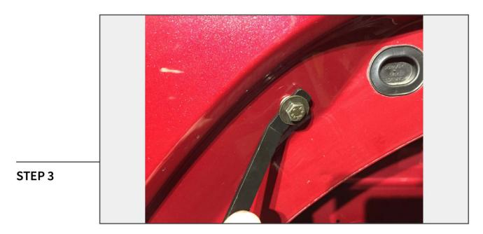
Using the supplied handle and long M6 x 1.0, install the rivnuts. Hold the rivnut in place with the handle and tighten the rivnut securing it to the vehicle. RIVNUTS ARE MORE SUSCEPTIBLE TO STRIPPING, DO NOT OVER TIGHTEN THEM.
