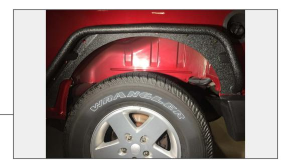
Install the M6 x 1.00 25mm bolts with the supplied washer and lock washer on all locations with the installed rivnuts.
