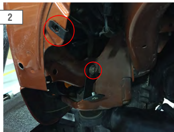
2 Remove the factory 10mm bolt and loosely install the supplied "L" bracket. Then slide on the supplied clip nut.
