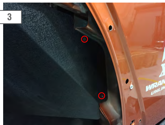
3 Loosely install the inner fender liner using the supplied Allen bolts. Using a marker, mark the hole locations on the rear most holes. These will need to be drilled. Remove the fender liners. Tighten the factory 10mm nut now that the bracket is in the correct location.
