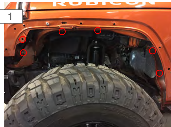
1 Locate the mounting locations on the fender well.
