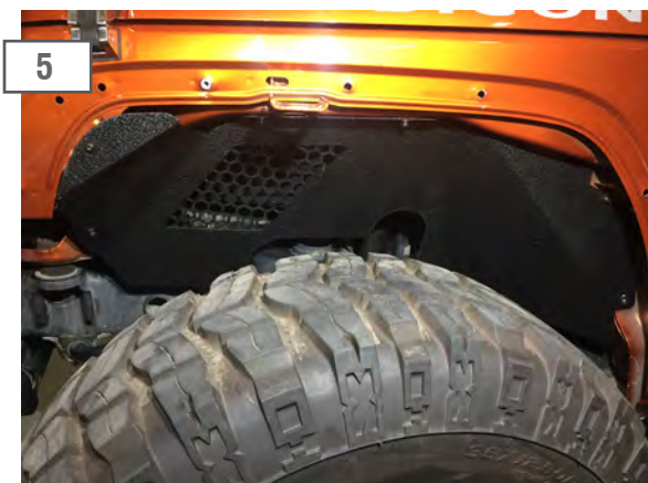
5 Install fender liners using the supplied bolts, lock washers, and large washers.
