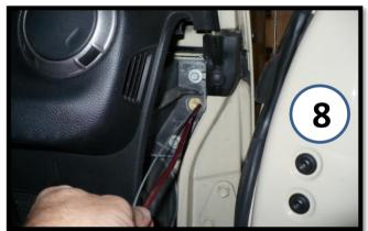
Behind it is a little hole that has foam in it. Use a piece of wire such as a coat hanger with the power wire taped to it and poke it through.
