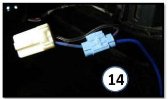
Tap into the blue wire with pink stripe. The Black/White Stripe wire is the Ground and remains as-is. Note: if you're adding other amplifier(s) for other audio upgrades, you only need to run this single Remote wire over to the amp(s) and can then splice into it for additional short runs to the other amp(s).
