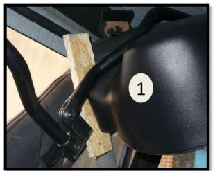
**Getting a feel for where it will go -** use a small piece of wood that's 1/2" thick to show how close the JKU-Pod should be to the downward sport bar. Place the wood as shown in the photo so it spans that side of the pod appropriately. Wood piece should butt up against fabric & metal; any factory wiring under the fabric should be moved aside.
