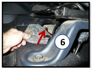
Amplifier Ground: An easy connection is already right under the Driver seat. It's up by the inner seat bracket on the uphill slope of the floor. Use 10mm wrench to loosen the nut and use a ring terminal on the ground wire. <u>Ground Wire must be connected to amp prior to</u> <u>attaching Power or Remote Wires to amp!</u>
