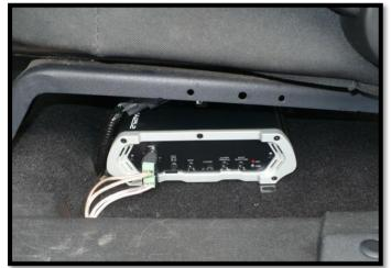
A clean looking install of the Kicker amp under the driver seat with only the speaker input leads showing. Easy access to amp's controls from here, and all other wires are on other side of amp and hidden from view.
