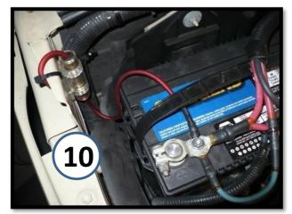
Fuse holder can be mounted by battery as shown. Don't connect the power wire unless amp ground wire is already connected so amp is grounded!
