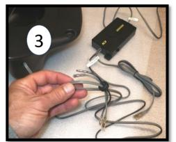
Then push the labeled 'Mid' wires through the grommet *in the opposite direction*. It's a tight fit but that minimizes air escaping the pod.
