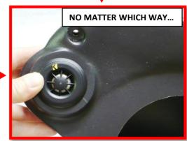
Flush or angled, you'll want the tweeter logo positioned at about the angle seen here (driver side pod) for final install. (Mirror image position for passenger pod.)
