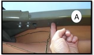
In these photos with the foam piece removed, you can see where the screws will enter the sport cage on the driver side. (Mirror image for passenger side.)
