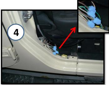
If you don't have an aftermarket radio and are tapping into the factory sound bars' speaker wires for signal, do it here by the passenger seat. The wires are under the plastic trim. Pop out the two plastic rivets and remove some of the electrical tape. Your wires will go under the carpet . Follow the wire color code below, making sure to mark which is which for the amp.
