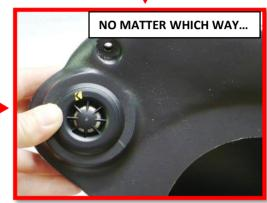
Flush or angled, you'll want the tweeter logo positioned at about the angle seen here (driver side pod) for final install. (Mirror image position for passenger pod.)
