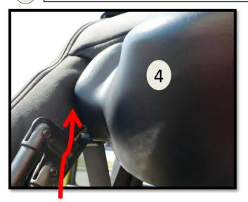
Prior to screwing the pod in place, you must decide how to get the speaker wires under the fabric. 1) You can run them through the factory opening for the soft top bars with a small amount of wire showing, or 2) you can use a razor blade and cut a tiny slit in the fabric right next to the grommet hole so the speaker wires exit the pod immediately going under the fabric. If choosing that way, hold the pod in place, determine where the slit should be made, remove the pod and make the slit.
