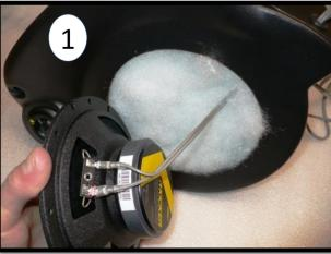
Re-install the poly-fill and connect the 'Mid' wires to the woofer.
