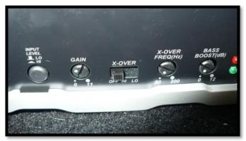
For Kicker amp, this is how we ended up setting ours: Stock 130 radio in our Jeep so input level is on High and we tapped into the sound bar speakers. We put the gain about a third of the way up and kept the x-over off so the pods get the full audio spectrum. We had the bass boost down/off. We had our regular stock 130 radio set at +4 bass, +1 treble, +2 mid, balance centered and fader at +4 Front. It's at least a good starting point for you if you got the Kicker amp too.
