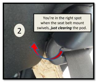
With the ½" wood spacer in place, you can tell the pod is at the correct angle when the seat belt guide (shown) can swivel past the pod, missing it by just a little bit. (If it's missing it by more than ¼" you need to swing the pod forward).
