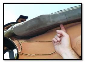
These two photos show you where the screws will penetrate the foam and affix the driver side pod. (Think mirror image for the passenger side.) The foam can sort of jiggle around, but that goes away when the pods are installed.
