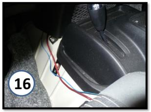
Bring the Remote and Amp Power wires under the carpet, between driver seat and center console so they can come up from under the carpet under the driver seat. You can bring them up where the other factory wiring for the seat exits, or cut slits in the carpet exactly where they will need to be for the amp.
