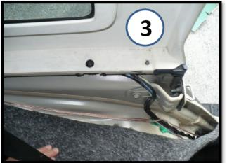
Continue running the speaker wires under the carpet along the driver side wheel well. Bring them under the rear floor carpet until you get under the driver seat. They can exit at seat bracket or you can make a slit in carpet at the exact spot where they'll connect to the amp.
