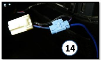
Tap into the blue wire with pink stripe. The Black/White Stripe wire is the Ground and remains as-is. Note: if you're adding other amplifier(s) for other audio upgrades, you only need to run this single Remote wire over to the amp(s) and can then splice into it for additional short runs to the other amp(s).
