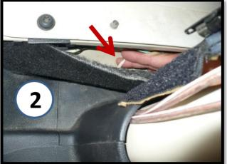
Pulling the carpet back, you can grab the wires as they're fed under the plastic piece at the base of the sport bar.
