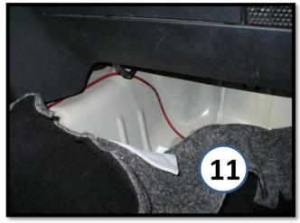
Run Power Wire under carpet in passenger foot area and feed it under center of dash on top of metal hump until it exits over in the driver foot area. Leave it there for now and let's move on to the amp's **Remote Wire**.
