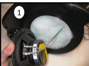
Re-install the poly-fill and connect the 'Mid' wires to the woofer.
