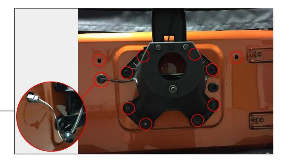
Start by removing the spare tire. Remove the rubber spare tire bumpers. Remove the 3rd brake light grommet from the vehicle and unclip the plug. Remove the (8) bolts holding the factory spare tire mount to the vehicle.
