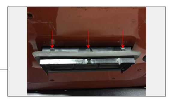
Once the factory mount is out of the way, use a small screw driver or panel removal tool to apply downward pressure the on the tabs highlighted above. To remove, push down and pull the vent off the vehicle.
