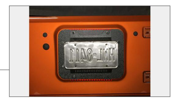
Install the license plate braket on top of the back plate. With the bolts loose, align the brackets so that they are flush with each other on the top and bottom. Then tighten all bolts.
