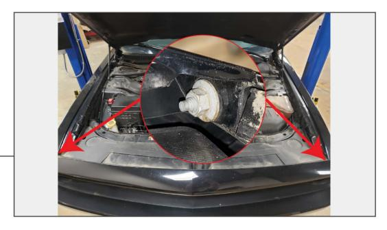
Locate and remove the (2) 10mm nuts securing the top of the bumper to the fenders, (1) on each side.
