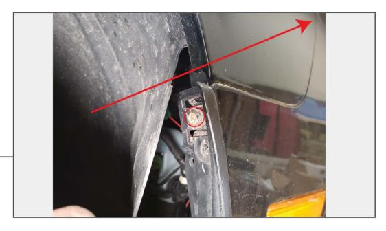
Fold back the fender liner and remove the (1) 10mm bolt and (1) 10mm nut securing the bumper cover to the fender.
