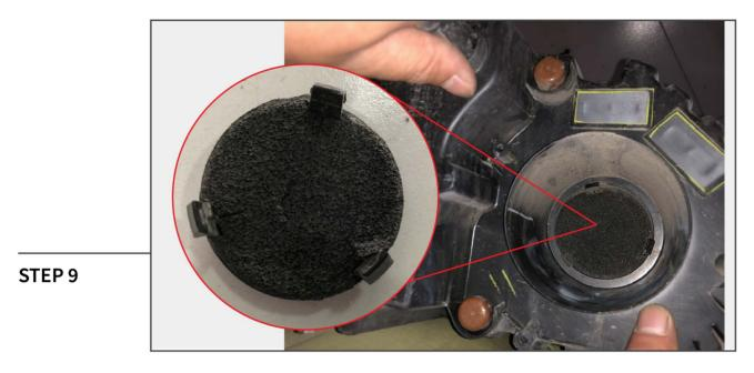
Remove the headlight plug. It is clipped in with (3) tabs, use pressure on the back of the plug to press it out of the light.
