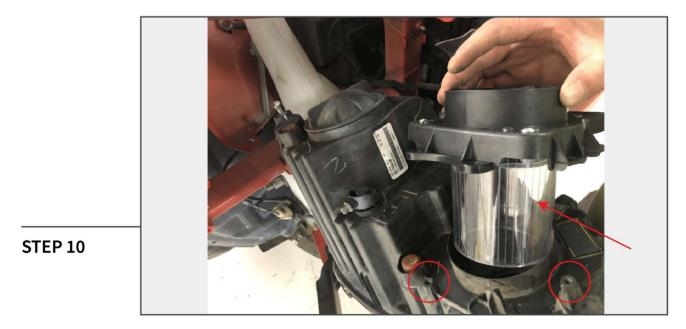
Install the light insert into the headlight. Secure it to the headlight using (3) Phillips screws into the factory light bosses.
