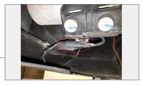
With a helper, locate and remove the fog light wiring connection. Disconnect this plug and then carefully remove the bumper from the vehicle.
