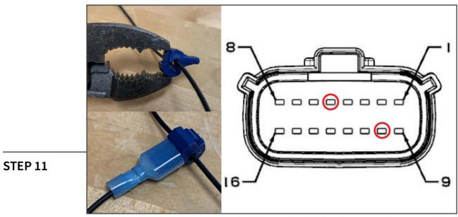
Wiring Instructions: Wire the headlight insert into the factory headlight plug using the supplied scotchlok and male spade connectors. Using pliers, squeeze the scotchlok connector onto the factory wiring. Crimp the male spade connector onto the headlight insert wiring. Then, insert the spade connector into the scotchlok connector. \*\*Note the photo is looking into the plug. The wires will be coming out he opposite side.
