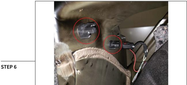
Pull back the left and right trunk liner to access the back of the tail lights. Remove the (2) plastic twist nuts.
