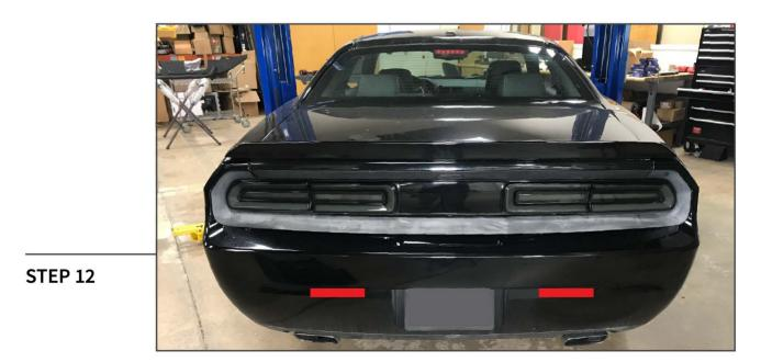
Complete the installation by installing the supplied reflective tape on either side of the license plate.
