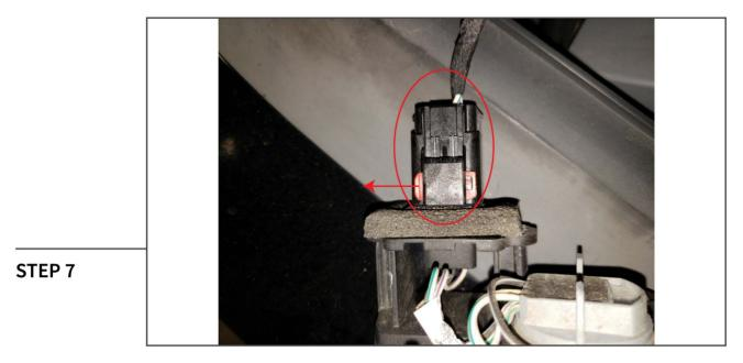
Carefully pull the tail light away from the vehicle for easier access to the electrical connector. Slide out the red locking retainer. Then depress the plugs tab and pull it away from the light.
