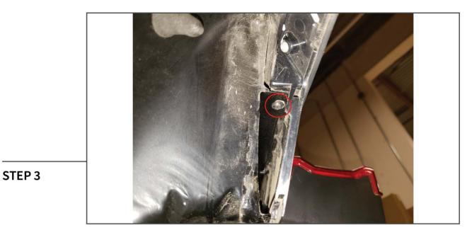
Using a Phillips head screw driver, remove the screw located behind the trim panel. There is (1) on each side of the center tail light.
