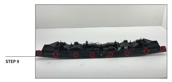
Using a Phillips head screw driver, remove the screws securing the factory tail light trim to the factory tail light.
