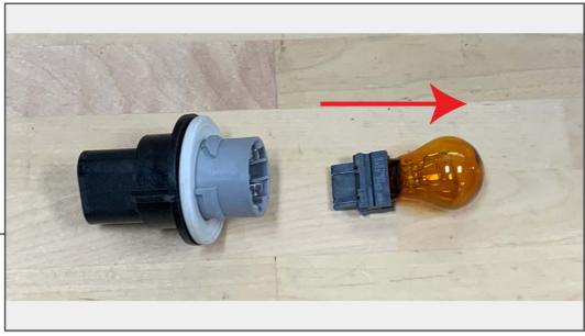
Turn the factory turn signal socket counterclockwise and remove it from the factory light. Remove the factory bulb by pulling it out of the socket.
