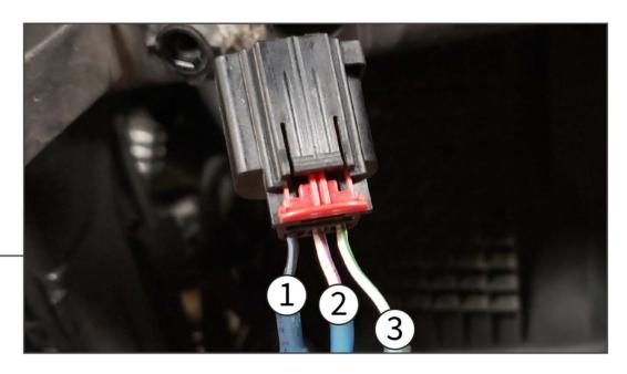
Splice the accent wiring into the factory (3) wire headlight plug as follows:
