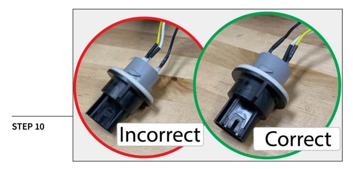
Insert the LED plug from the new headlight into the factory socket. Note the orientation of the wiring to the light socket. If the LED plug is backwards, the light will not operate correctly. Insert the turn signal socket into the new headlight. Twist the socket into the headlight housing to lock it into plate.
