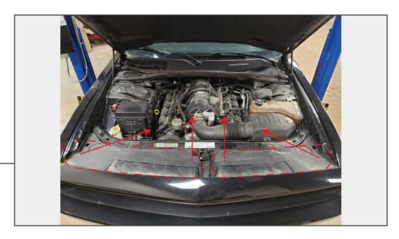
Begin by raising and supporting the front of the vehicle using a jack and jack stands. Open the hood and remove the radiator trim panels. Pull the panels up in the center and then away from the fenders.
