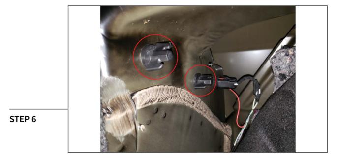
Pull back the left and right trunk liner to access the back of the tail lights. Remove the (2) plastic twist nuts.
