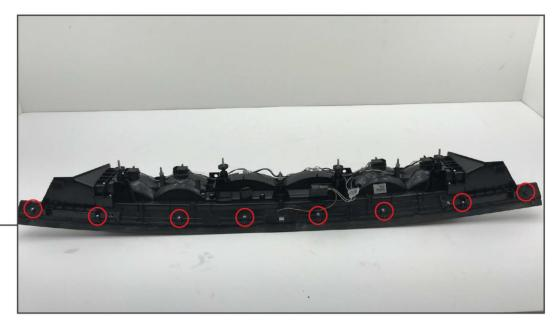
Using a Phillips head screw driver, remove the screws securing the factory tail light trim to the factory tail light.
