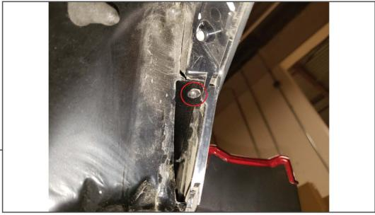
Using a Phillips head screw driver, remove the screw located behind the trim panel. There is (1) on each side of the center tail light.
