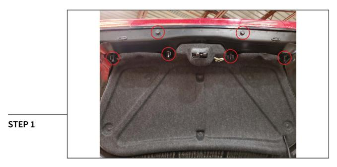
Begin the installation by removing the (4) plastic twist nuts and (2) bump stops located on the trunk lid.
