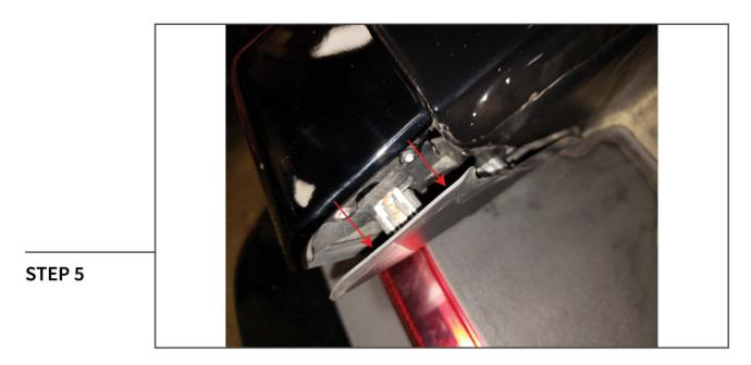
Using a soft pry tool remove the left and right side tail light trim panels.
