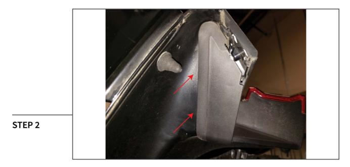
On either side the of the trunk lid, use a panel removal tool to pry off the tail light trim cover.
