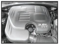
Step 2 Remove the engine cover.
