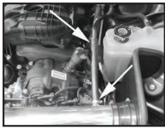
Step 18 Connect the breather hose to the existing plastic vent line, then to intake tube. Once in desired position fasten securely in place.
