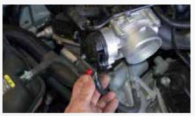
Unplug the electrical connector from the side cover of the throttle body. Pull the black wire harness mount out of the hole in the throttle body.
