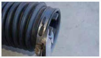
The stock air inlet tube will work with the BBK throttle body. Just open the clamp all the way up before installing. Trim off the 2 small tabs on the top of the stock rubber inlet tube so it will fit all the way onto the BBK throttle body. A little WD-40 or light grease may help this process.
