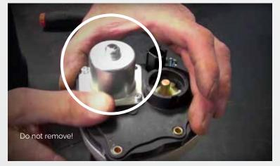
Install the motor housing minus the removable cap onto the BBK throttle body over the plastic spring cap and tighten screws.
