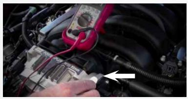
With your meter still connected, loosen the mounting screws on the TPS sensor and gently rotate it until the desired voltage is achieved, then tighten the screws.
