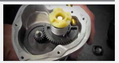
Be sure that the plastic capped spring is hooked into the gear and rotated approx 180° COUNTER-CLOCKWISE until it pops into locked position.
