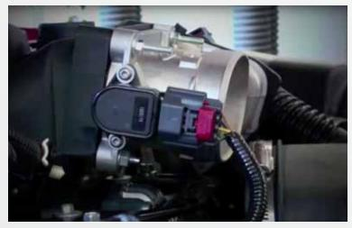
Unplug the throttle body electric motor, TPS, and mass air meter by sliding the red colored locking clips back, and then squeezing the tabs on each wiring connector while pulling them from their connections.
