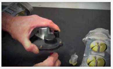
Pop the removable circular cap off of the motor housing. (This is easily done with a finger or tool).
