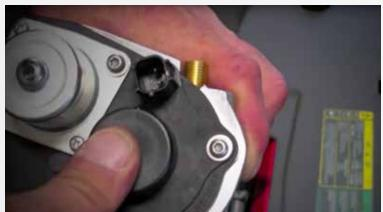
Align the tabs on the removable cap with the slots on the motor housing and snap it into place.
