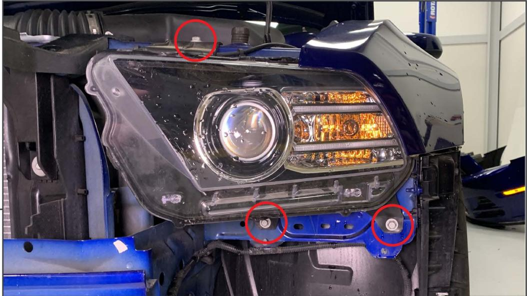
Remove (3) 10mm bolts from the vehicle headlight assembly. Pull the headlight away from the vehicle and disconnect the (2) electrical connectors.
