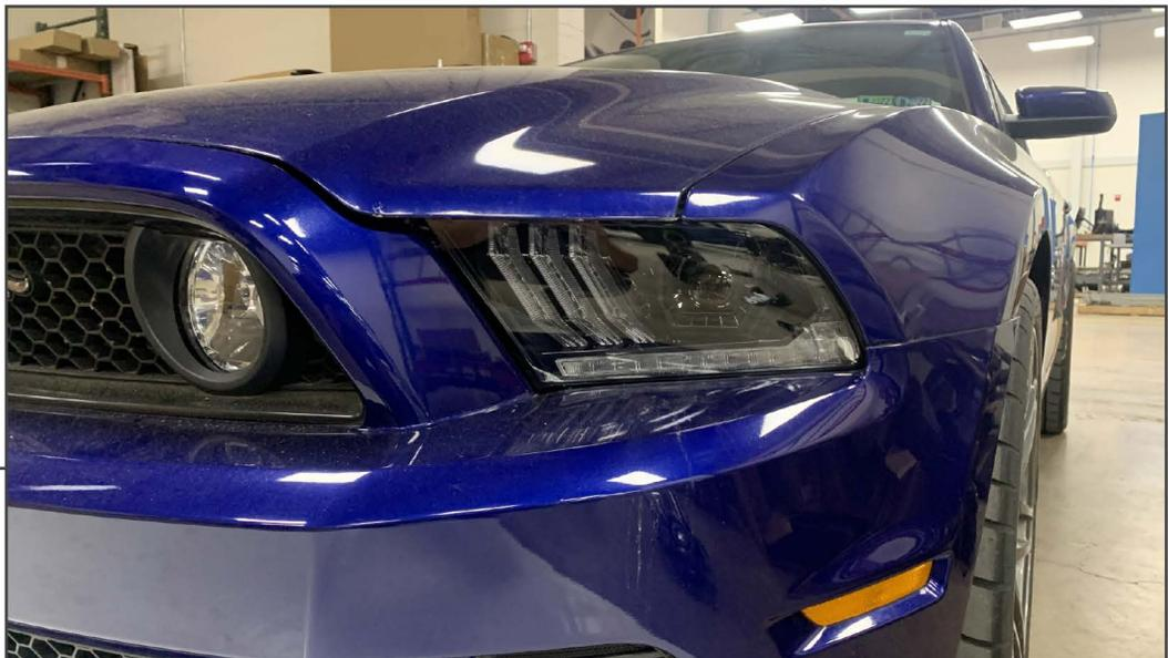
Install the new headlight to the vehicle using the original (3) 10mm bolts, test functionality. Once tested, re-install the bumper to the vehicle following steps 1-4 in reverse order, re-using the original hardware.
