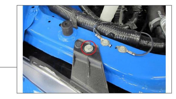
Remove (1) 10mm bolt from the top of the headlight in the radiator support. Pull the headlight from the vehicle and unplug the (2) electrical harnesses.
