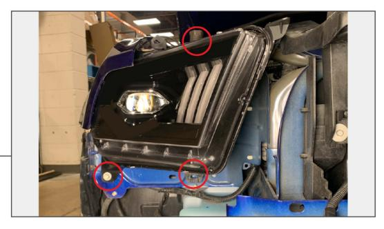
Secure the new headlight into the vehicle reusing the (3) original 10mm bolts. Tighten until secure.
