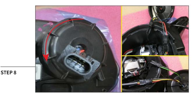
With the headlight assembly unplugged, determine if the vehicle has OEM halogen OR OEM HID headlights by inspecting the electrical connector (3 Wires = OEM Halogen / 4 Wires = OEM HID).
