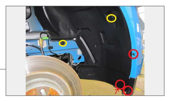
Lift and support the vehicle using a jack and jack stands. Remove the wheel from the vehicle. Remove (3) 7mm screws and (2) plastic push clips from the inner fender liner.
