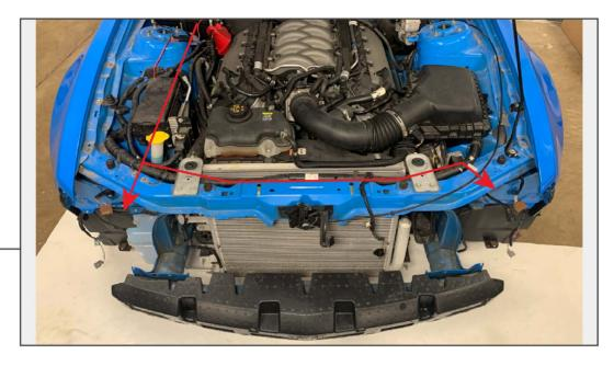
Route the provided (1) DRL harness neatly across the engine bay. Ensure the power/ground leads are routed towards the RH side of the vehicle. Connect the wire leads to the vehicle battery terminals.
