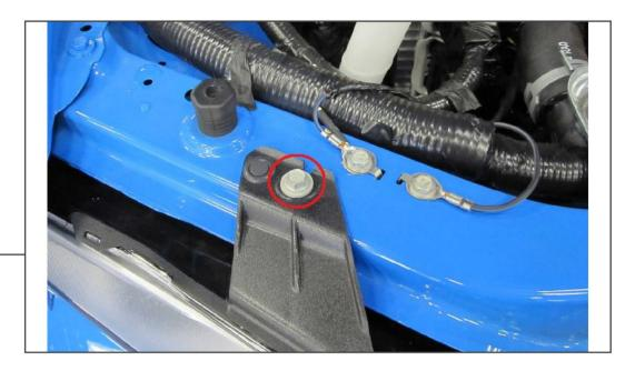
Remove (1) 10mm bolt from the top of of the headlight in the radiator support. Pull the headlight from the vehicle and unplug the (2) electrical harnesses.
