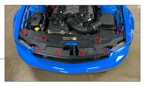
Remove (8) plastic push clips using a panel removal tool. Lift the radiator support cover from the vehicle and set aside.
