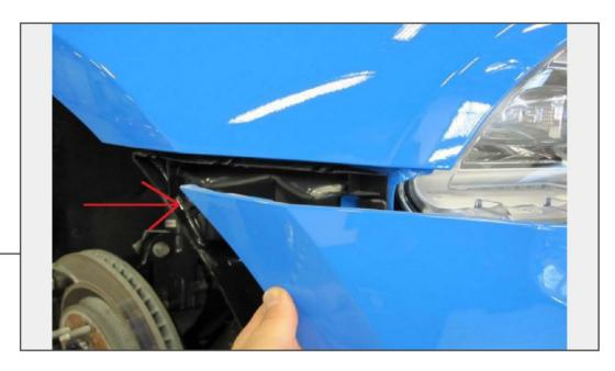
Grab the corner of the bumper where it meets the fender, and firmly pull forward to allow the bumper to separate from the fender on both sides of the vehicle. Disconnect the side marker light connectors and fog light connectors. Lift and set bumper aside carefully to prevent damage.
