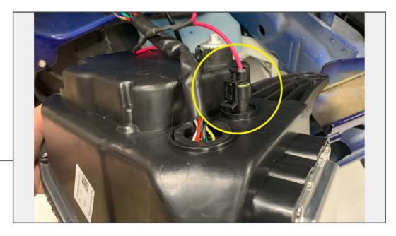
Plug the DRL harness into the backside of the headlight assembly. Plug in the (2) headlight wiring harnesses into the corresponding vehicle harness. Ensure the connectors click into place secure the connection. Repeat this procedure for the opposite side of the vehicle.
