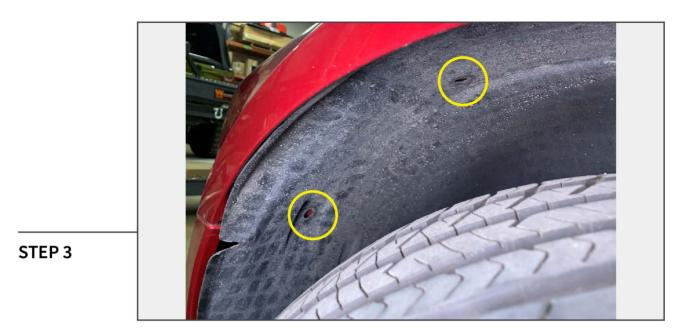
Remove (2) plastic push clips from the inner fender liner.
