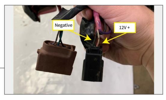
Splice the (2) additional wires into the vehicle parking light harness following the diagram below. Tap into the vehicle harness using (2) scotchlok connectors per side.
