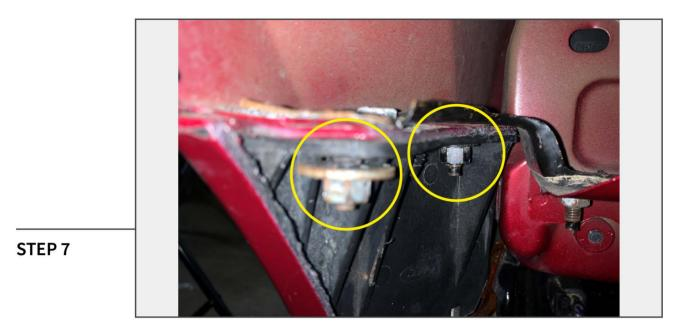
Remove (2) 10mm nuts connecting the bumper to the fender.
