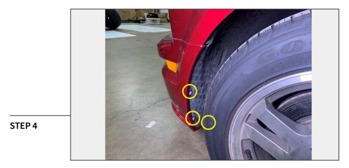
Remove (3) Phillips screws connecting the front bumper to the inner fender liner. Repeat this procedure to the opposite side of the vehicle.
