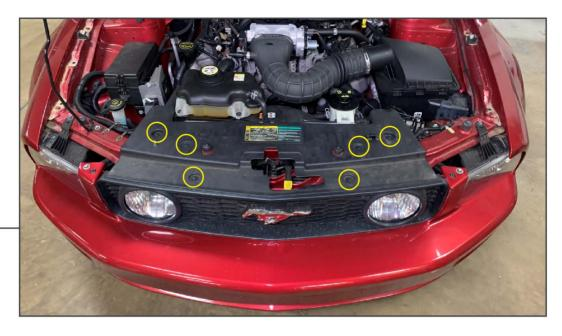
Open the hood. Remove (6) plastic push clips from the radiator support plastic cover. Remove cover from vehicle.
