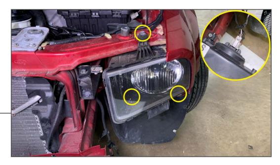
Remove (3) 10mm bolts from the headlight assembly. Remove the headlight assembly and disconnect the electrical connector.
