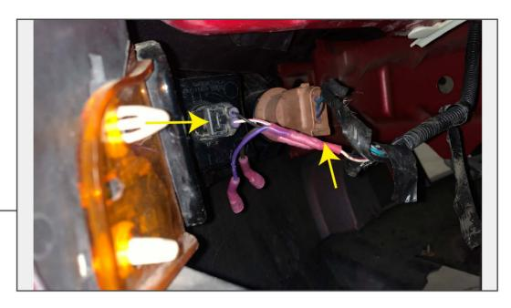
Reach towards the vehicle turn signal/parking light lens from inside the bumper and disconnect the (2) electrical connectors. Depress the plastic tab and pull the connector from the light socket.
