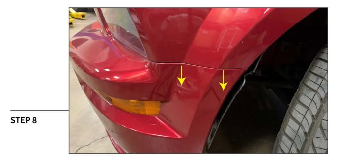
Pull downward on the bumper to dislodge the bumper from the fender studs, then pull the bumper outward.
