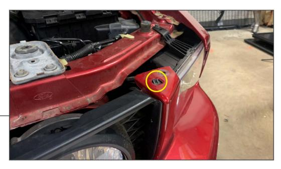
Lift the bumper over the mounting tab.
