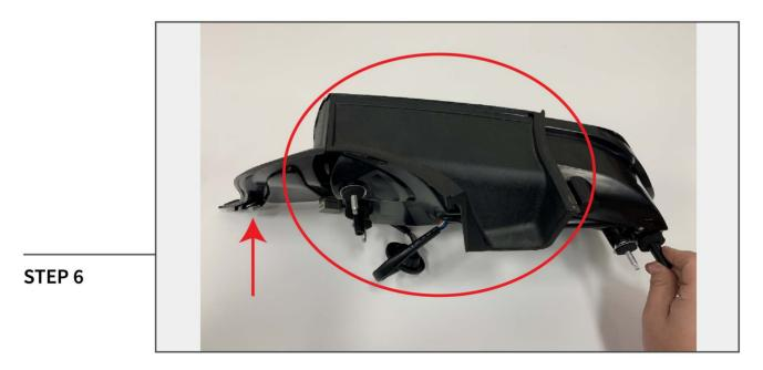
Install the top plastic cover to the new tail light housing.
