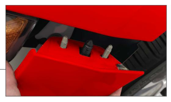
Firmly pull the edge of the bumper down to dislodge the clip holding the bumper to the fender. Lift the bumper away from the vehicle and place on a soft surface.
