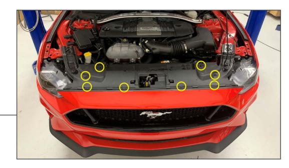
Open the hood. Remove (8) plastic push clips from the radiator cover. Remove the radiator cover from the vehicle.
