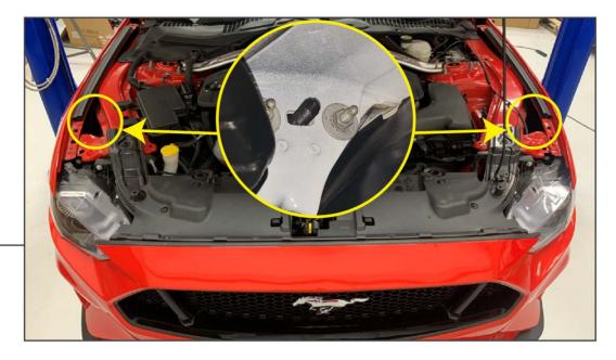
From the top of the vehicle, remove (2) 10mm nuts along the inside of the fender.
