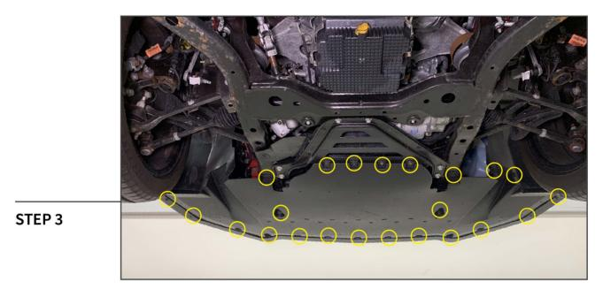
Raise and support the vehicle using a jack and jack stands. Remove the fasteners securing the splash shield to the vehicle. Remove splash shield from the vehicle.
