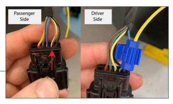
Using the provided ScotchLocks, splice the (1) additional wire into the vehicle headlight harness following the diagram below.
