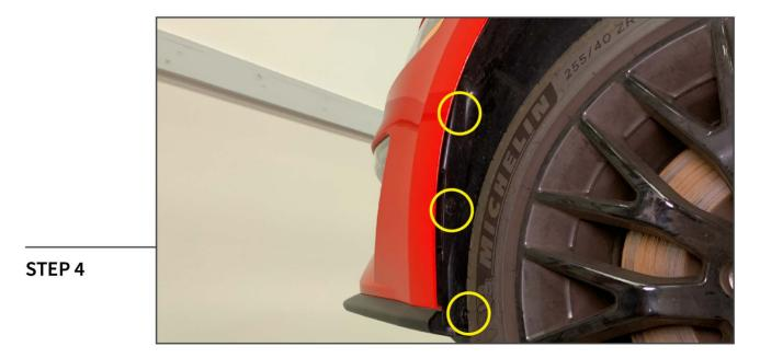
Remove (3) plastic clips on the fender liner on both sides of the vehicle.
