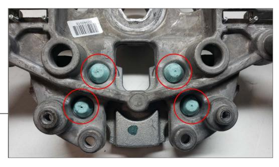
Carefully pry the weighted bracket from the factory steering wheel. Transfer weighted bracket to the new steering wheel by using needle nose pliers to pull the rubber inserts through the aluminum frame. Reinstall the plastic trim removed in step 6.
