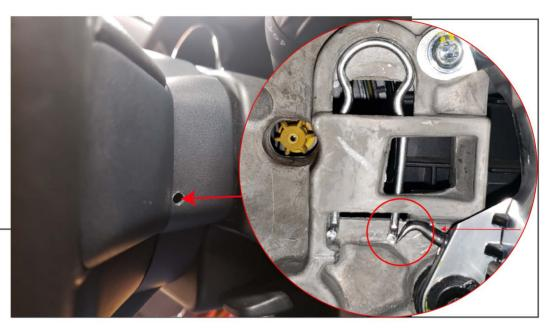
Begin by disconnecting the battery terminals, failure to do so could result in deployment of the airbag. Next, insert a pick, small flat head screwdriver, or Allen key into the holes located on each the side of the steering wheel. Press the tool into the hole to release the airbag retaining clip. This will release the airbag from the steering wheel.
