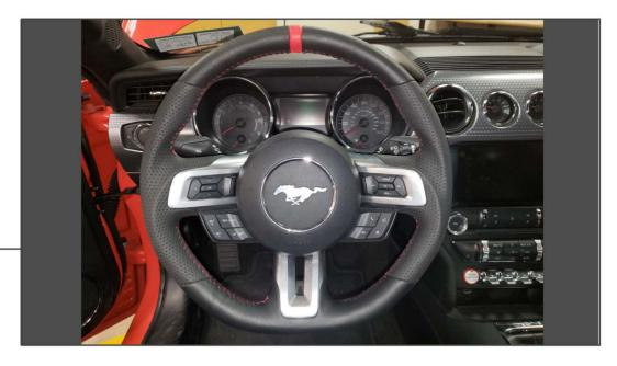
Install the steering wheel in reverse order. Torque the 24mm steering wheel nut to 35 ft/lbs. Reconnect all electrical connections before pressing the airbag back onto the steering wheel. Finally, reinstall the battery terminals to compete the installation.
